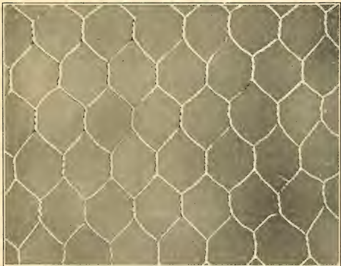
Wire Netting. Darker Wires Show Rust. Rusted While in the Roll
