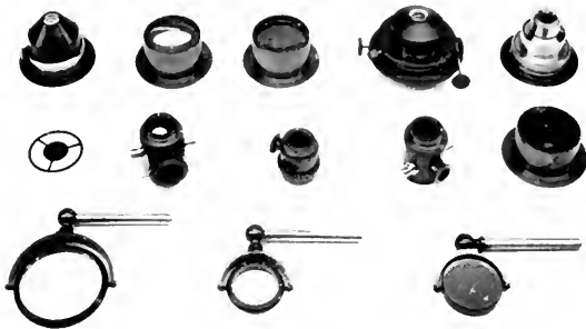
Fig. 7 - Condensers and illuminators used in microscopy
