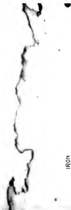
Fig. 4. The application of high-power photography to the study of nickel finishes. One of the characteristics of an improved process for plating ductile nickel on iron is the interlocking or "keying" of the nickel and the iron. Magnification, 6000 X.
