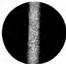
(b) Coloring matter in glass. The glass was colored saffranin and was transparent to the eye or with any other method of microscopic vision but with the slit ultra-microscope the colloidal coloring matter becomes visible. Also taken with the Lucas photomicrographic camera, a time exposure being necessary. Magnification, 100 X.
