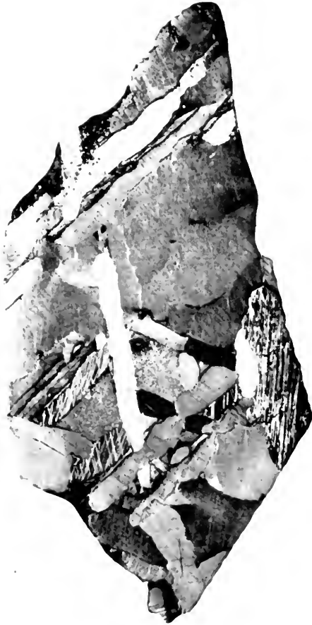
Fig. A. Meteoric iron consists of iron, nickel and the other elements usually found in steels, such as carbon, sulphur, phosphorus, etc. The study of meteorites has contributed much valuable knowledge to the science of metallography. The Widmanstätten figures (shown by the arrangement of the constituents with reference to crystallographic planes) were generally considered characteristic of meteoric iron and it was believed that they were not to be found in manufactured iron and steel. Later this was shown to be an incorrect view.
