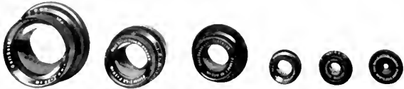
Fig. 4—A battery of low-power lenses. These lenses are used without eyepieces. Each lens is equipped with a diaphragm for stopping the aperture.
