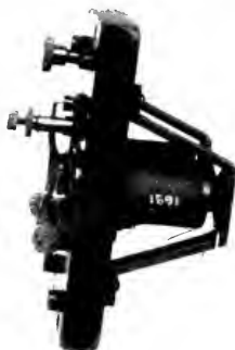
Fig. 3—Early telegraph relay used as telephone drop
