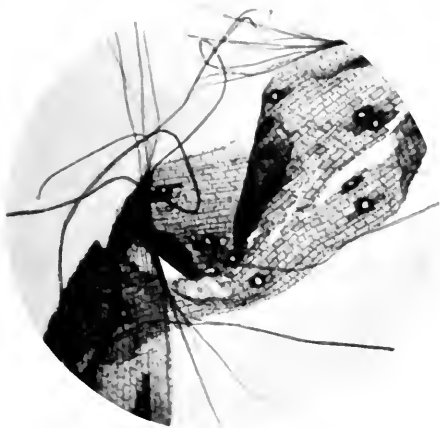
Fig. 11. Manila hemp rope is used extensively in telephone work and the fiber from old rope is used in paper for cable insulation which finds its way into the plant.
