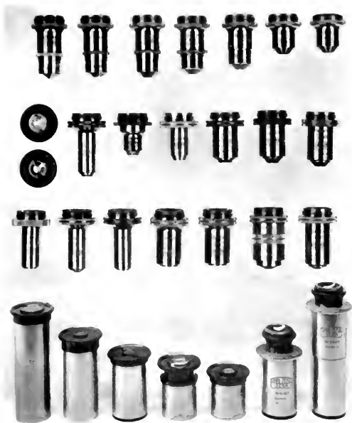
Fig. 5—A battery of medium and high-power objectives and eyepieces
