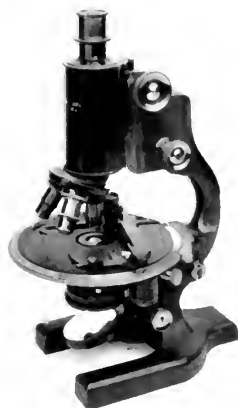
Fig. 3—Research type of microscope by Spencer Lens Co. Large barrel for photo-micrography; a large revolving stage with graduated circle, and a removable mechanical stage.
