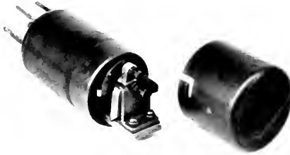
Fig. 7 Early supervisory relay
