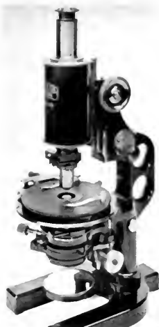
Fig. 2—Research type of microscope by Zeiss. Large barrel for photo-micrography; revolving mechanical stage, and sliding objective changers.
