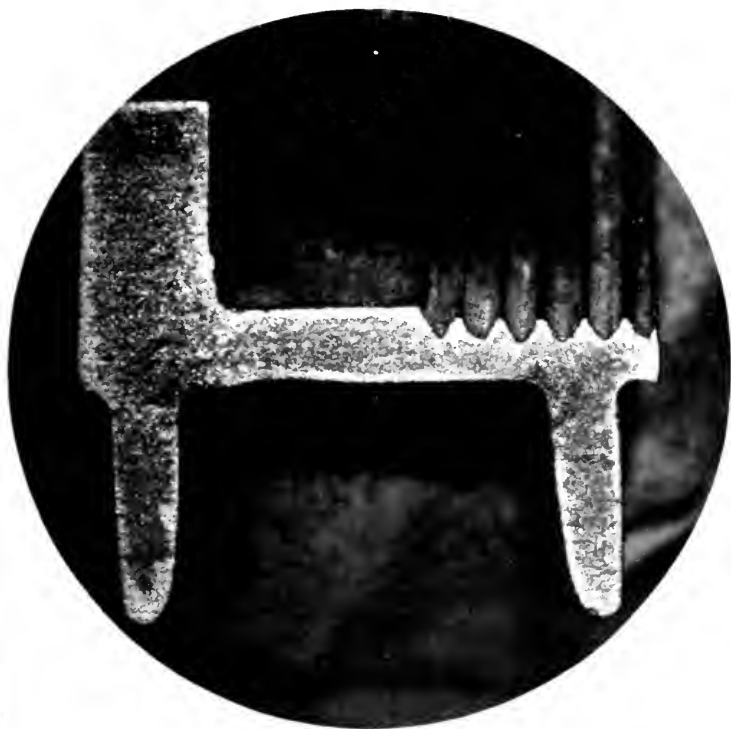
Fig. 1. (a) Faulty pack hardening of truck wheels on ball truck distribution system. The object of pack hardening is to impart a highly carburized wearing surface to the otherwise soft steel part. The interior remains soft and ductile. Lack of uniformity in hardening or insufficient depth of the carburized zone causes soft spots which result in unequal wear. The magnification is 112 X.
