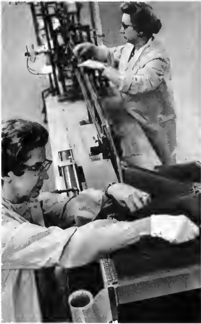
An important part of every Electronic Switching System is the memory unit. This one is being assembled at the Hawthorne Works in Chicago.
