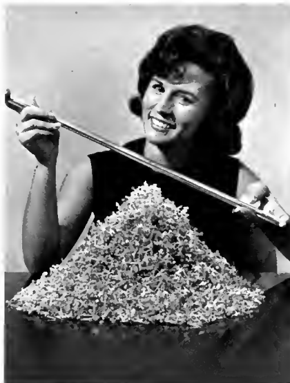
The 20-inch rod held by Linda Smith of Western Electric's Allentown, Pa., works is $1,500 worth of pure gold. It is used in plating 10,000 transistor parts such as those heaped in front of it. Western Electric uses gold on transistors and other devices it manufactures for the Bell System because of the metal's electrical properties and the qualities that make it resistant to corrosion and easy to join to other metals.
