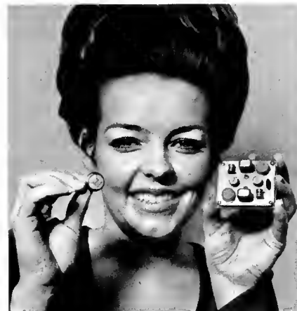
The minute device resembling an earring is a monolithic crystal filter which now does the same job of controlling frequencies in the telephone network as the equivalent conventional filter on the right. Developed at Bell Telephone Laboratories, it is being produced by Western Electric.
