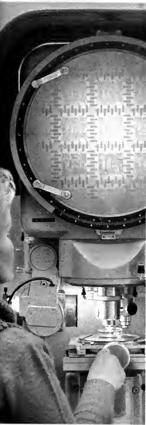
Integrated circuits are magnified hundreds of times at the Allentown Works to check quality.
