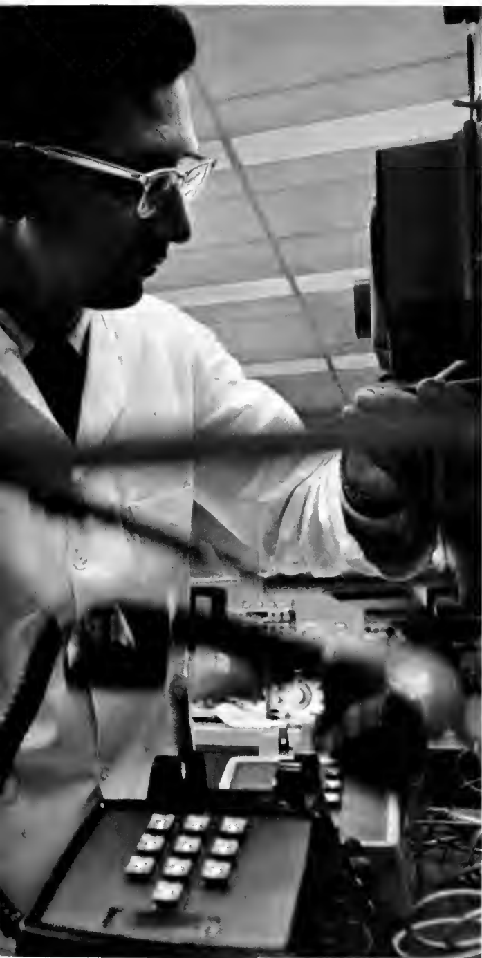
Telephone receivers are simultaneously removed and hung up during one of the endurance tests run by Western Electric to insure that Bell System phones will be as trouble-free as possible.
