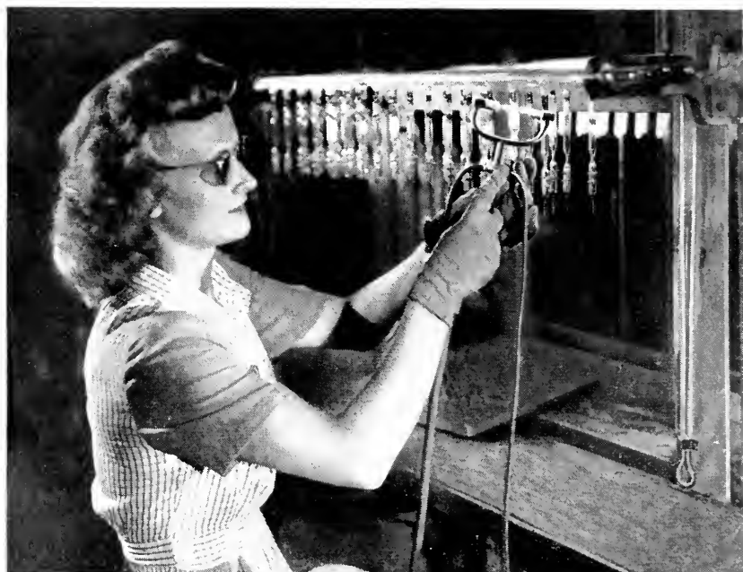
Fig. 35—Pump Station for the 724B Vacuum Tube
