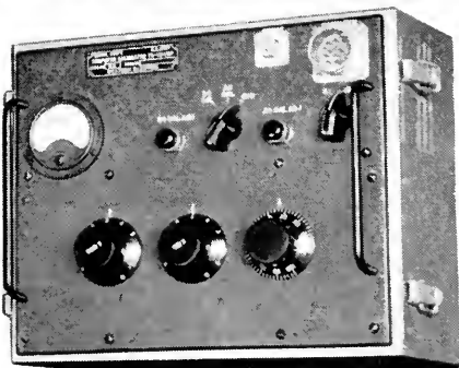
Fig. 28—Two test sets for checking the computers used in bombsight and fire control radars.
