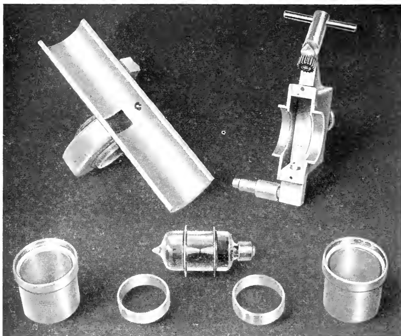
Fig. 7—Exploded view of the cavity of Fig. 6
