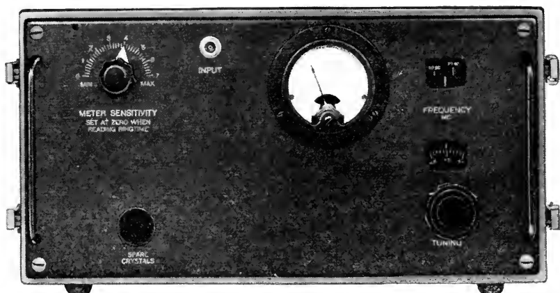
Fig. 14—Panel view of a 9 kmc echo box.
