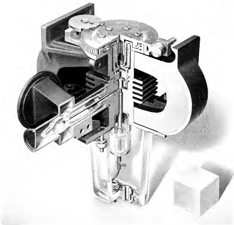
Fig. 71—A view of a sectioned 2J51, tunable, "packaged" magnetron (55 kw., 8500 to 9600 mc/s). Features of interest to be seen are: the tuning pins, the drive mechanism and vacuum bellows, the axial cathode mount, the glass bead support of the center conductor of the coaxial output line, and the sheathed permanent magnet construction.
