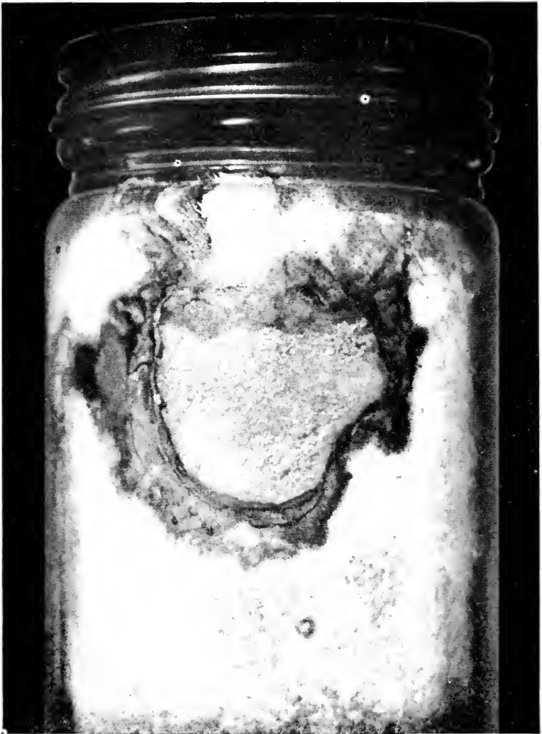
Fig. 6—Antagonism which has persisted for over one year between the wood-destroying fungus, Lentinus lepideus (outer portion) and contaminating fungus (inner portion) in a soil culture.
