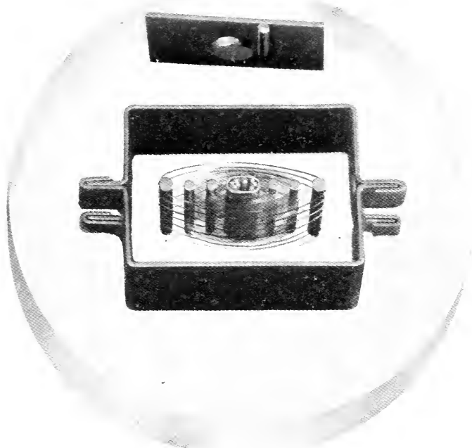
Fig. 13—Transverse section of 6AK5 tube ( 5\frac{1}{2} times).
