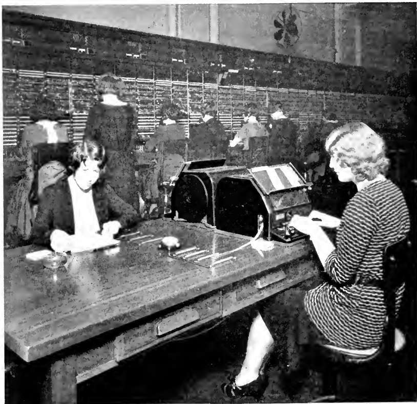
Fig. 2—Transatlantic telephone operator's position showing arrangement of printing telegraph equipment.
