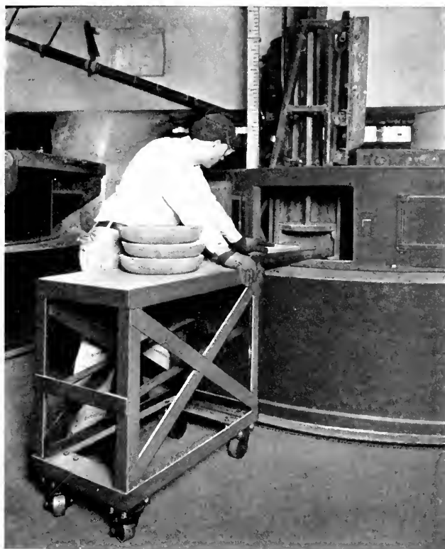
Fig. 27—Antimony charging mechanism.
