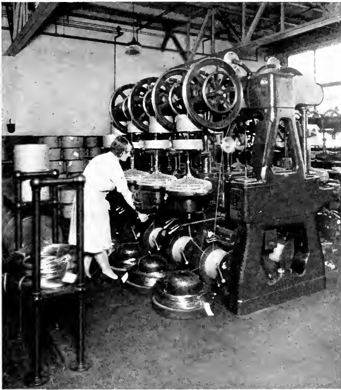
Fig. 6—Paper insulating machine.
