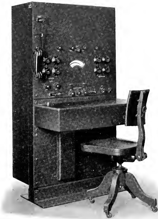
Fig. 31—D.C. insulation resistance test desk—front view.
