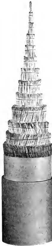
Fig. 4—Typical construction of long distance telephone cable.
