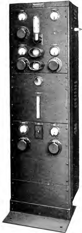
Fig. 3—Front view of crystal controlled oscillator-amplifier unit.
