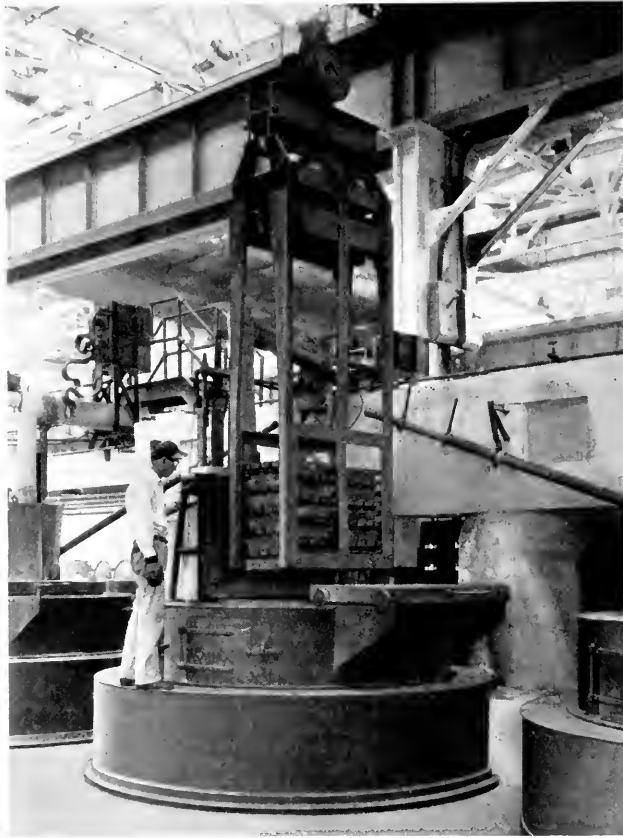
Fig. 26—Charging of lead-melting kettle.
