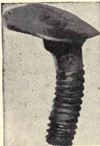
FIG. 103.—Worn Bolt from Lagging of Conveyor Pulley.
