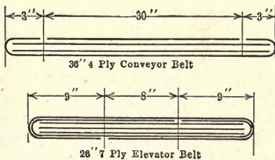
FIG. 50.—Assembly of Duck to make Certain Belts according to Metcalf's Specification.
