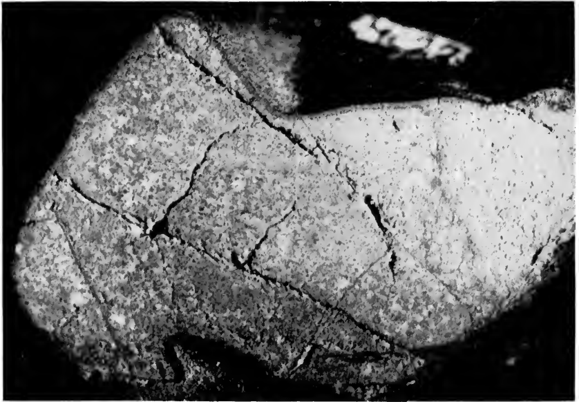
FIG. 73. Polished section showing crustal zones; metallic (left) and black (right) veins; and cracks; \times 2.5 .
