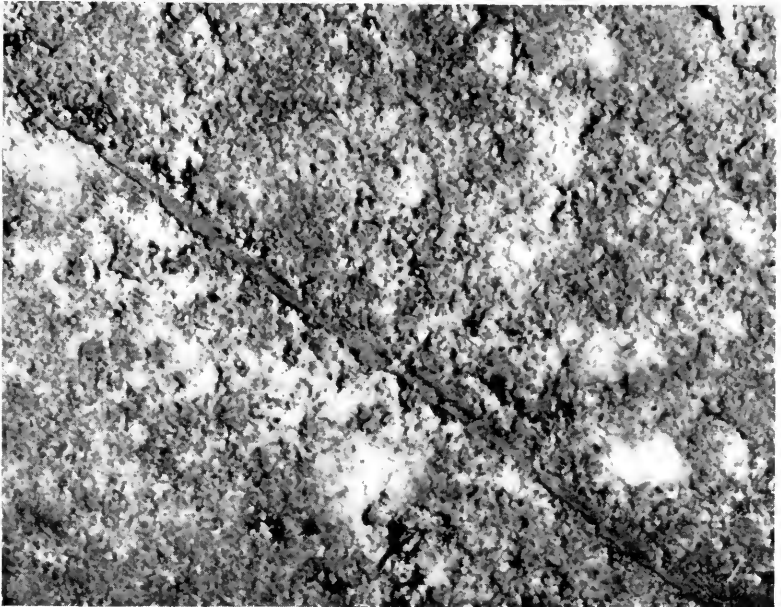
FIG. 75. Enlargement of the metallic vein shown to the left of figure 73; \times 8 .
