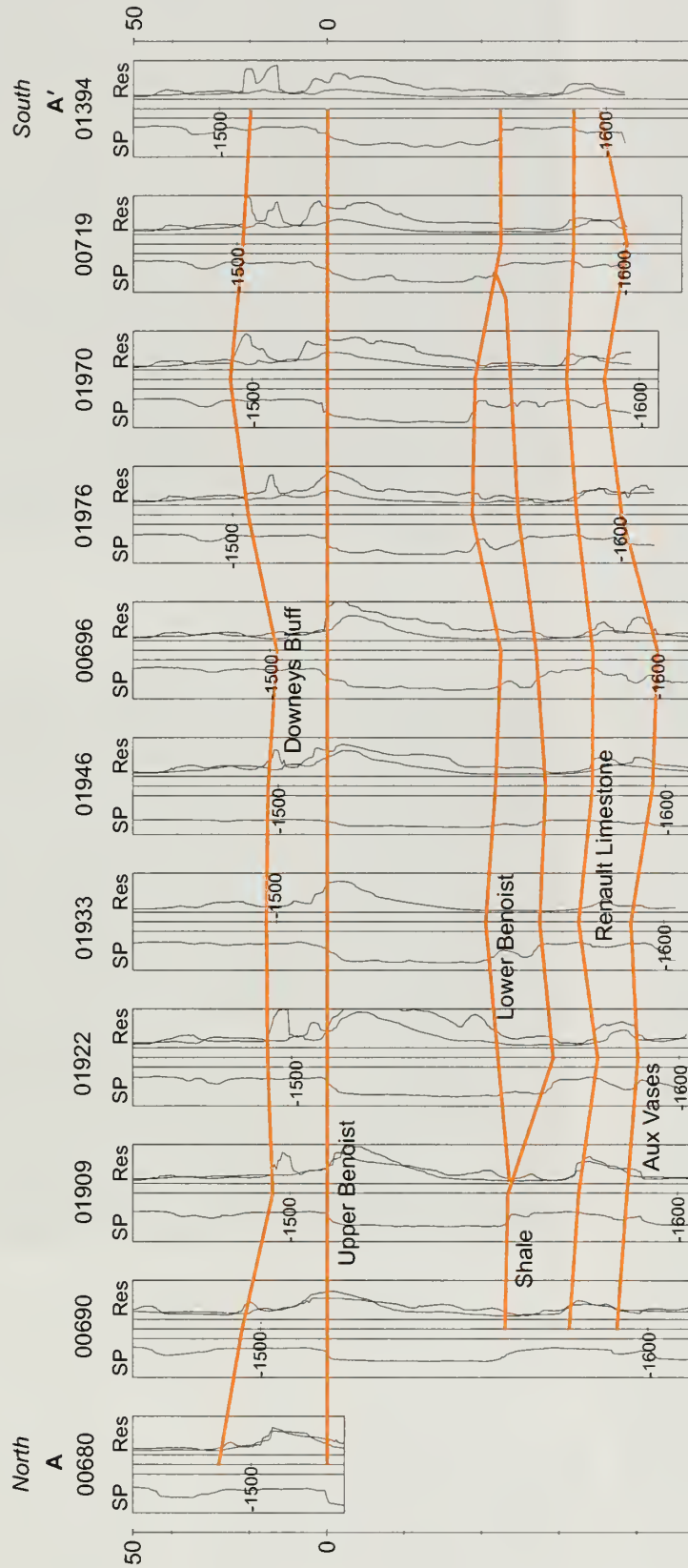
Figure 13 Cross section A-A' showing the thickening and thinning of the Benoist interval. The line of cross section is shown in figure 6.
