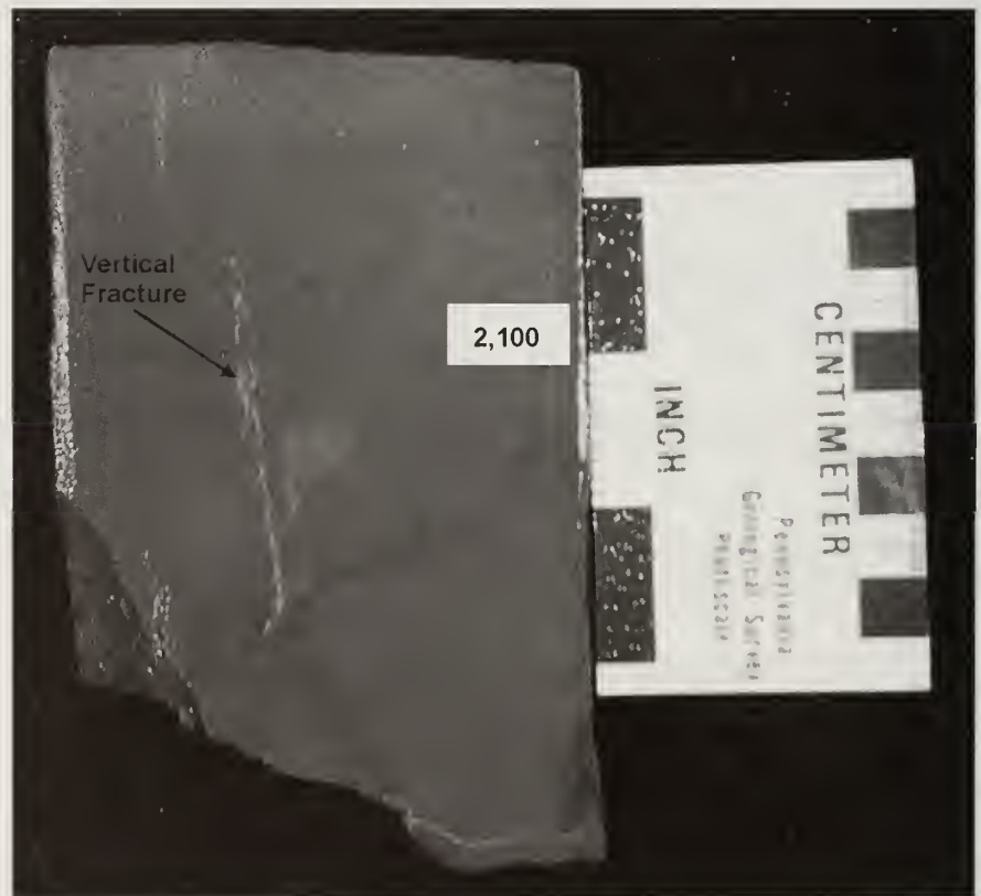
Figure 24 Photograph of Benoist sandstone core from Boyd Field showing a vertical fracture extending most of the length of the core. The white-colored material along the fracture is calcite cement. Superior Oil Company, Shallert No. 1 well, 2,114 feet.
