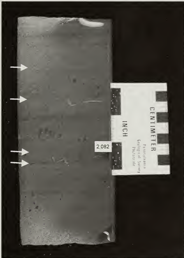
Figure 9 Benoist reservoir sandstone showing shale laminae (arrows) that may impede vertical fluid flow through the reservoir. Superior Oil Company, Schallert No. 1 Well, 2,082 feet.
