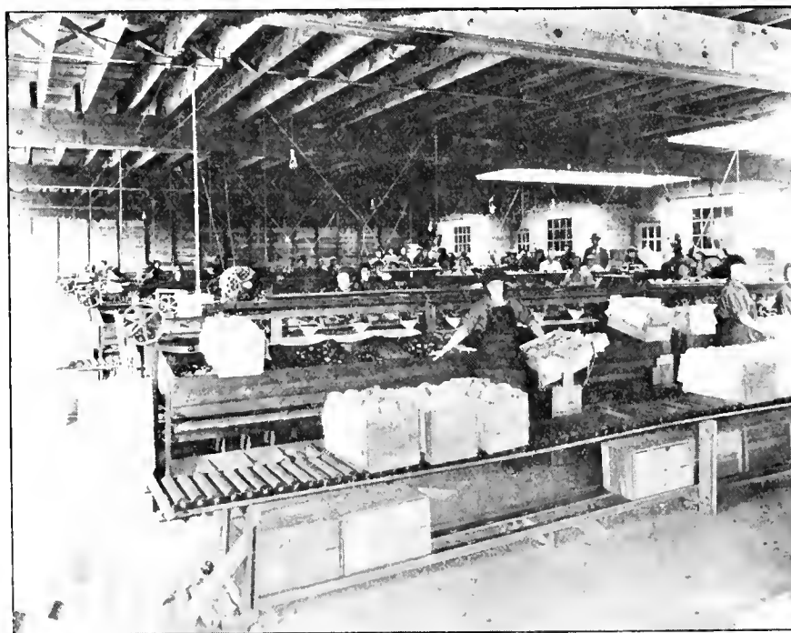
Scene in typical apple packing-house showing four big, motor driven grading machines and practical application of gravity conveyor. This unit can turn out an average of 4000 boxes a day easily.
