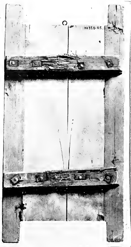
15. Wooden Mould for Making the End Plate of a Five- or Six-Plate Stove.
