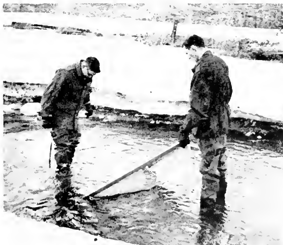
Staff collects river bottom organisms and the organisms found are identified and typed. This determines the degree of river pollution
