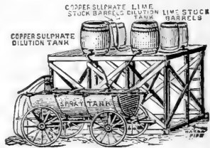
ELEVATED PLANT FOR MAKING BORDEAUX ON A LARGE SCALE
