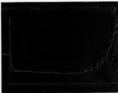
FIG. 2. Typical record of the course of hemolysis of ox blood in 2M ethylene glycol. The time intervals are 5 seconds with every twelfth signal omitted.
