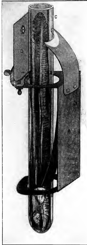
FIG. 20a. — Leeuwenhoek's Mechanism for Examining the Circulation of the Blood.
