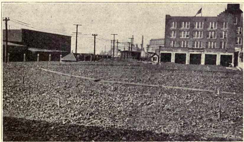
FIG. 1. PILE OF SCREENINGS WITH TEMPERATURE TUBES, CLOSED AT UPPER ENDS BY WOODEN PLUGS
