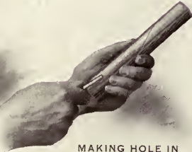
MAKING HOLE IN SIDE OF CARTRIDGE
