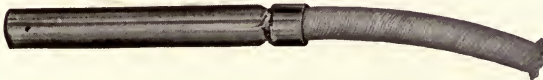
BLASTING CAP CRIMPED ON FUSE WITH A DU PONT CAP CRIMPER No. 3
