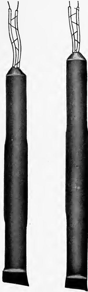
First and Second Delay Electric Fuzes (Actual Size)
