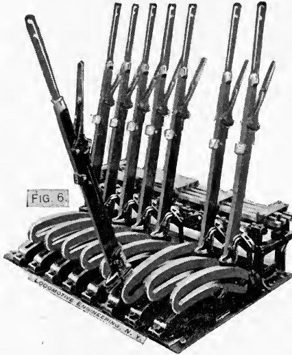
THE IMPROVED SAXBY & FARMER INTERLOCKING MACHINE.
