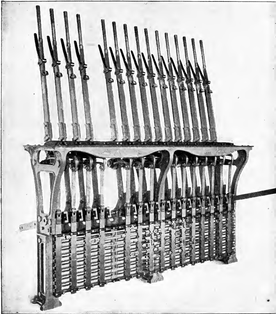
FIG. 1.—THE NATIONAL INTERLOCKING MACHINE.
