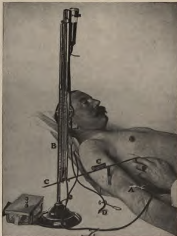
FIG. 68.—The Moritz-Tabora venous blood-pressure apparatus: A , cannula in vein; B , manometer scale; C , level; D , escapement. (After Hoffmann.)
