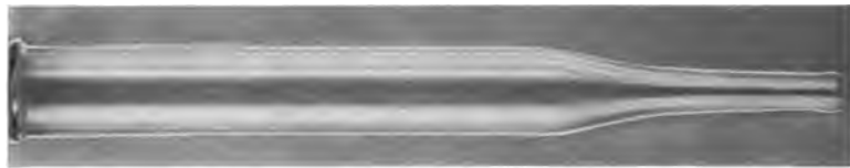
FIG. 1.—Flanged glass nozzle.
