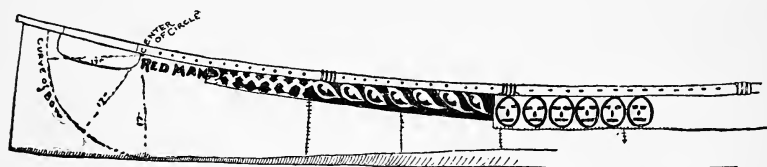
Fig. 95.—Shows how to describe arc of circle for bow, also ornamentation of winter bark.
