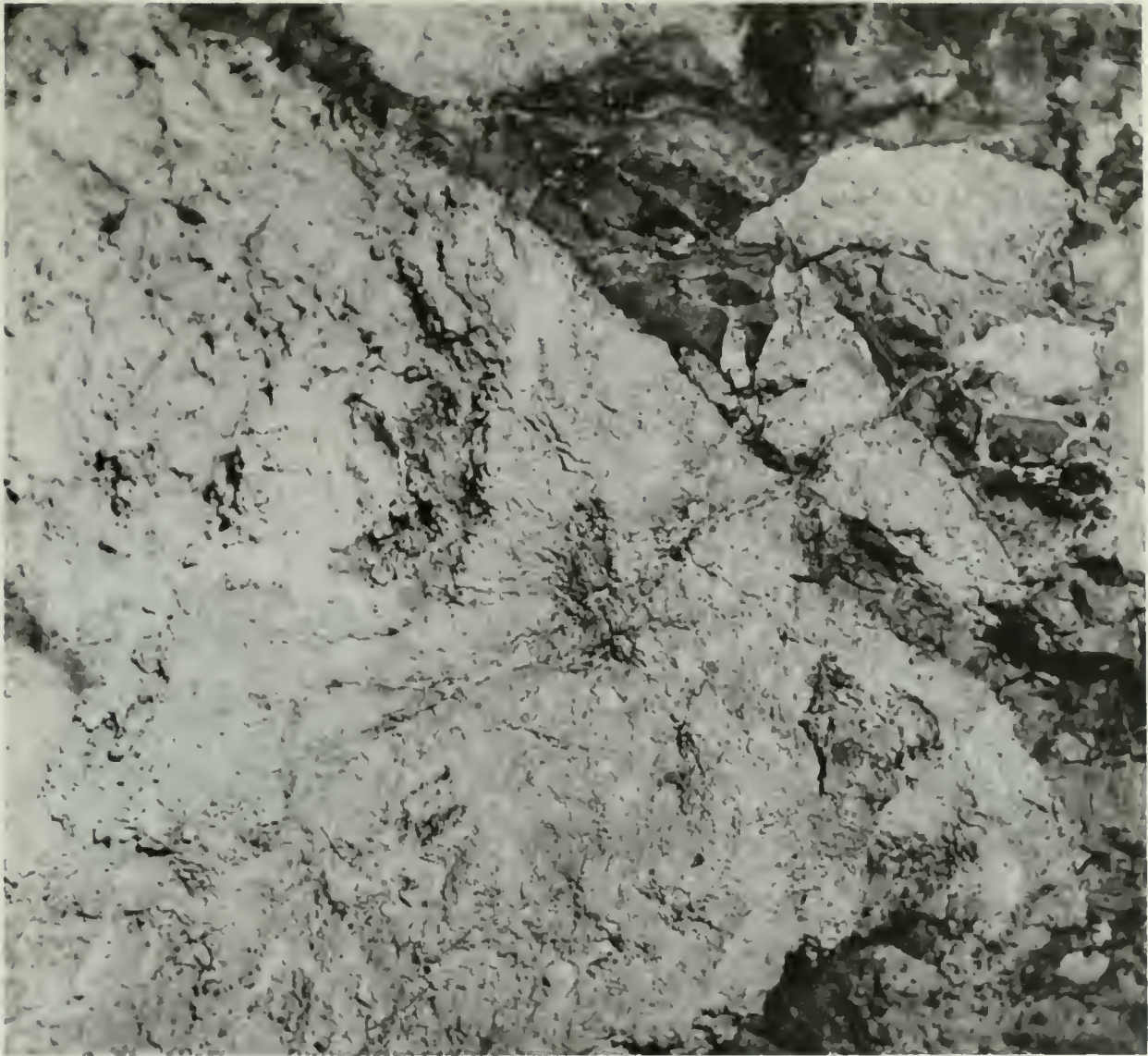
Photo 14. Argillically altered tuff breccia of the Silver Hill Volcanic Series, cemented by dark gray, pyrite-rich chalcodony. 700 level of the Red Cloud mine. Photograph by Francis H. Frederick.
