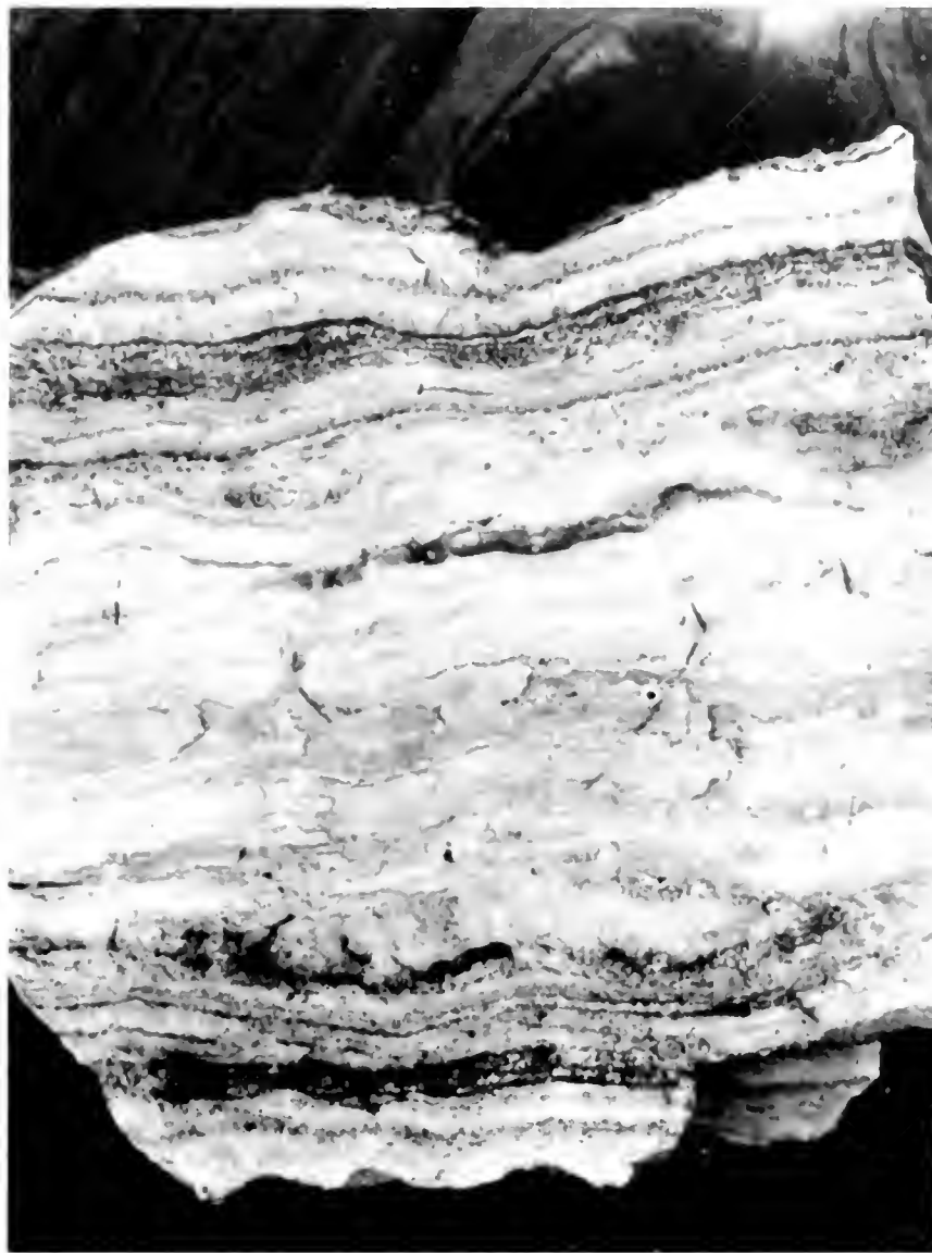
Photo 9. Ribbon quartz, containing fine-grained free gold. Typical of the veins mined in the Bodie Bluff area. Photograph by Francis H. Frederick.
