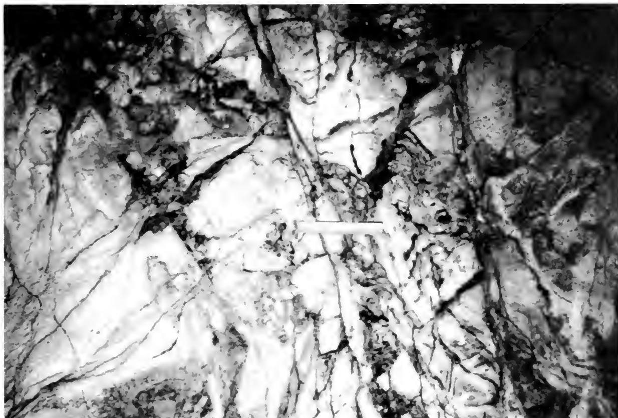
Photo 8. Fractured and propylitically altered intrusive dacite of the Silver Hill Volcanic Series, as exposed underground in the Bulwer tunnel, about 50 feet from the contact between the intrusive dacite and tuff breccia. Scale is 6 inches long and lies across a quartz vein that dips steeply to the right.
