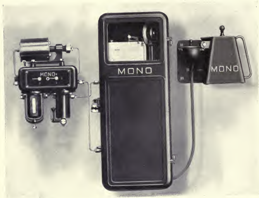
FIG. 7.—Original "Mono" automatic gas analysing machine for CO and unburnt gases only.
