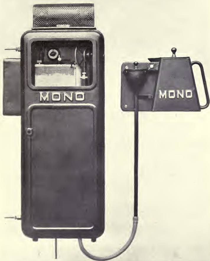
FIG. 4.—“ Duplex Mono,” closed as when working normally in the firehole.
