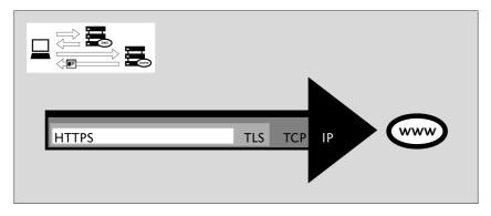
In the above example, the HTTPS protocol relies on the **TLS** protocol to perform encryption of the communications so that they are private and unmodified as they travel across the network. The TLS protocol, in turn, relies on the **TCP** protocol to ensure that information is not accidentally lost or corrupted in transmission. Finally, TCP relies on the IP protocol to ensure that data is delivered to the intended destination.
