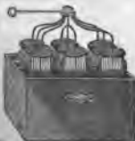
ELECTRICAL BATTERY. A primary sort of battery, as called from its power of pro-
