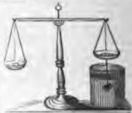
HYDROSTATICAL BELLOWS. A machine for showing the upward pressure of fluids, and the hydrostatical paradox.
