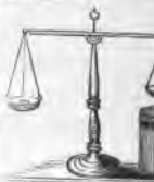
HYDROSTATICAL BALANCE. A machine for showing the upward and downward pressures of fluids, and the hydrostatical
