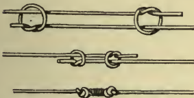
FIG. 68. THE STRONGEST KNOT FOR GUT-CASTS.
