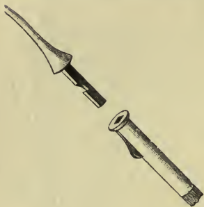
FIG. 14. METHOD OF FASTENING GAFF TO HANDLE.
