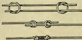
FIG. 15. THE STRONGEST KNOT FOR TYING LENGTHS OF GUT TOGETHER.
