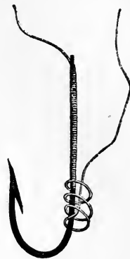
FIG. 10. FINISH OFF OF WHIPPING.
