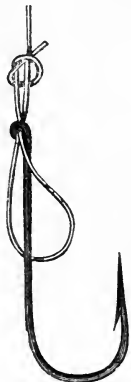
FIG. 20. KNOT FOR HOOKS WITH LARGE EYES, AND FOR LARGE FLIES.
