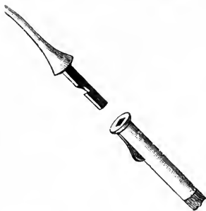
FIG. 14. METHOD OF FASTENING GAFF TO HANDLE.
