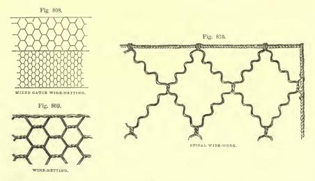
invented by Mr J. Reynolds, of 27 New Compton Street, Soho, London. It is made of hard twisted wire, galvanised after being manufactured. From the way in which the twisted wires are interlaced, no other fixing is required. This would make an ornamental fence against cattle and sheep at a farmhouse.
