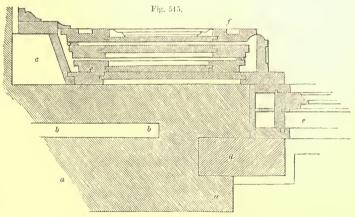
PLAN OF SHUTTERS OF WINDOW OF HOUSE IN FIG. (5-SCALF, 1 INCH TO THE FOOT.
