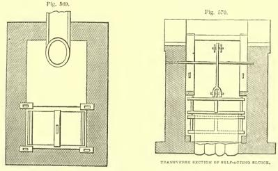
fig. 570 a transverse section of a self-acting sluice, designed by Mr Archibald Sutter, C.E., Edinburgh, and described by him in his valuable paper on
