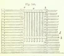
rods of iron e batted with lead into the wall, and with a shoulder and nut and The height in front should not exceed 2 feet 9 inches for screw in front.
