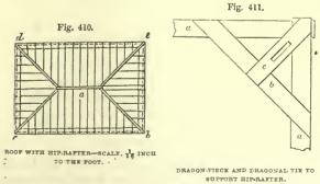
1212. Another method is to form a frame as a a, b c, fig. 411, which is placed at the corner of the walls. Upon this framing the lower termination of the hip-rafter is fixed, the upper resting on the king-post. Where a tie-beam is introduced, the
