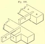
as c, fig. 190, should be carried up from the footings, on which to lay the flooring-joists d. This allows the air to circulate round the end of the joist,
