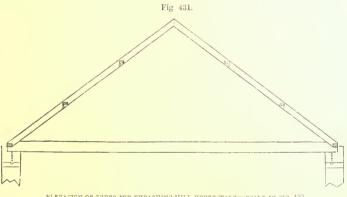
ELEVATION OF IRUSS FOR THRASHING-MILL HORSE-WAIK-SCALE IN FIG. 430.
