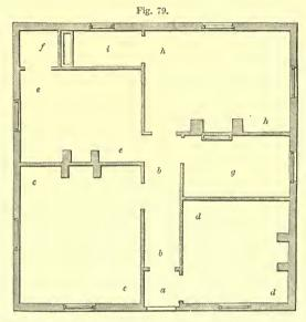
GROUND-FLAN OF A SINGLE-STOREVED DETACHED COTTAGE-SCALE, 1 OF AN INCH TO THE FOOT.
