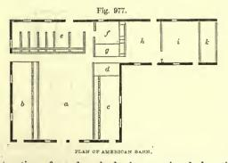
fig. 977, in which  $\alpha$  is the barn floor, 24 feet by 42; b cow-stable, 12 feet by 38, c 12 feet by 31; d oat-bin, 5 feet by 12; e workhorse stable, 14 feet by 32; f tool-room, 14 feet by 12; g wheatbin, 5 feet by 12; h colt-stable, 16 feet by 20; i calf-stable, 16 feet by 20; k corn-crib, 8 feet by 20. The height over the cowstables is 7 feet, over the main floor and horse - stable 9 feet. Fig. 603, p. 373, in the section
