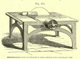
fast and loose pulleys cd; and the termination e is fitted to receive a boring bit f, fig. 3, which may be used for boring holes in timber. The timber to be cut is placed upon the table g, figs. 1, 2, 3, and 4, which can, by means of a screw h, fig. 4, be moved laterally parallel to the saw, so the thickness of cut can be easily adjusted, and to the greatest nicety. The timber to be cut is kept up to the action of the saw by the atten-
