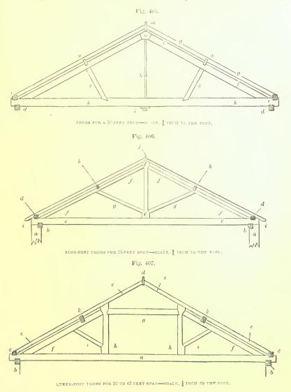
truss for a 30-feet span, but is adapted to spans from this extent up to 45 feet. The tie-beam is at a, 10 inches by 5; b b wall-plates, 6 inches square; c c pole-plates, 5 inches square; d ridge-pole, 8 inches by  $1\frac{1}{2}$ ; e c common rafters, 4 inches by  $2\frac{1}{2}$ ; f f principal rafters, 9 inches by 5; g straining-beam, 9 inches by 5; h h queen-posts, 7 inches by 5; i i struts, 5 inches square;
