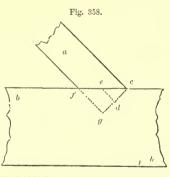
JOINT OF FOOT OF RAFTER WITH THE-BEAM-SCALE, 1 INCE TO THE FOOT.
