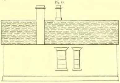
BACK ELEVATION OF A SINGLE-STOREYED DETACHED COTTAGE-SCALE IN FIG. 81.
