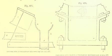
gutter-box, of cast-iron, secured to the wall-plate or column by bolts and nuts  $b \ b$ ;  $c \ c$  the rafters, secured to the angular pieces  $d \ d$  by bolts and nuts as shown. The rafters may be continued, as shown by the dotted lines, and secured by bolt and nut.
