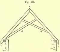
TRUSS FOR A PORCH-SCALE, \$ INCH TO THE FOOT.
