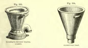
1116. Fig. 304 illustrates a very simple and cheap form of closet-pan. Fig. 305 represents a form of water-closet pan and trap formed in one piece, wholly of earthenware, so as to require no woodwork for its support. The top is spread out about four or five inches, so as to form a self-sustaining seat. The entrance of the pipe for carrying off the effluvia to a ventilating tube or chimney is shown at *a*. This form, when properly constructed, and with an ordinary service-pipe
