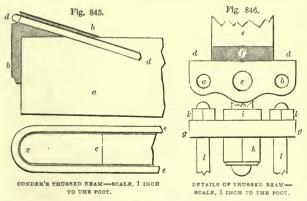
invented by Mr J. Conder, and described at p. 158, vol. i. of the *Engineers' and Mechanics' Encyclopædia*. The plan is applicable to the trussing of solid beams, that is, those which are not cut down the middle into two flitches. The general appearance of the trussed beam is that of fig. 841, the truss rods being on the outside of the beam, in
