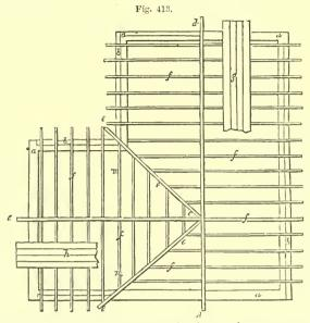
TIMBER OF A ROOF MEETING AT RIGHT ANGLES (PLAN)-SCALE, 1 INCH TO THE FOOT.
