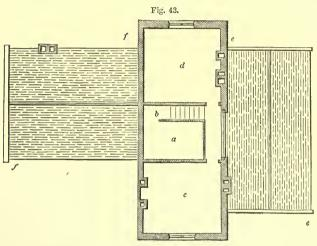
6 feet 6 inches wide; b stairs, 2 feet 6 inches wide; c servants' bedroom, 12 feet 9 inches by 12 feet; d second bedroom or storeroom, 12 feet 9 inches by 12 feet; e e plan of roof over apartments g and h in fig. 42; f f plan of roof over apartments a a, b, i, k, in fig. 42.
