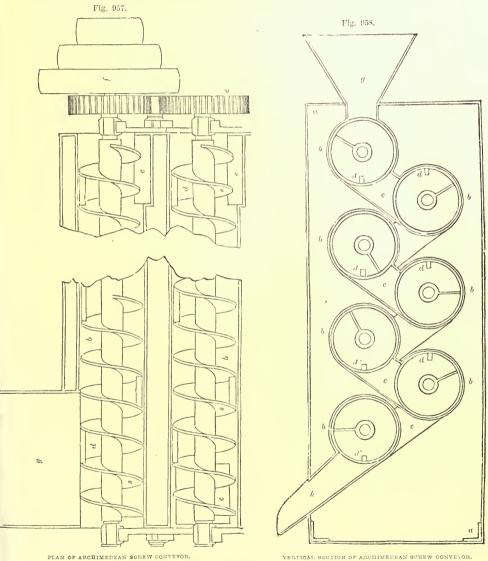
same, showing the communication of the tubes from one to another throughout the series. Fig. 959 is a detail representation, on a larger scale, of a portion
