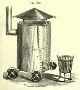
PERSPECTIVE VIEW OF ASPHALT CALDRON AND GRATE.
