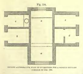
privy or water-closet, 3 feet by 6; c pig-sty, 4 feet by 6. Alternative Plan, fig. 133, in which a is the fuel-store, 5 feet by 6; b privy, 3 feet by 6; c pig-sty, 4 feet by 6; d a food-store, 3 feet by 6. Second Alternative Plan, fig. 134, in which the accommodation of cow-byre is given; a a the cow-byre, 18 feet by 6; b coalstore, 6 feet by 6; c watercloset, 3 feet by 6; d pig-sty, 4 feet by 6; e food-store, 3 feet by 6.
