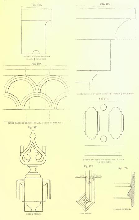
949. Stone Details of House in Fig. 45 in the Tudor-Gothic Style.—In fig. 171 we give an enlarged drawing of "finial" to apex of gable; in fig. 172, drawing of "drip-stone" to breakfast-room window, of which, in fig. 45, we give an elevation (and in plan at d d, fig. 41); and in fig. 173, section of mouldings of "string-course."
