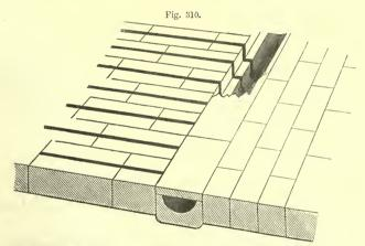
DRAINAGE PAVEMENT-BRIDES IN PERSPECTIVE, WITH GUTTER PARTLY UNCOVERED TO SHOW ITS CONNECTION WITH PAVEMENT.
