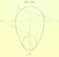
DESCRIBING AN ELLIPTICAL OR EGG-SHAPED DRAIN.
