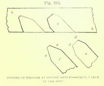
the beam f; *i* is a continuation of the beam f. An objectionable form of joint of this kind is shown in the right hand of fig. 357, where the beam a is joined to the beam b b by the tenon c passing into the mortise d.
