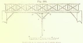
Fig. 561.  $\alpha$ h Ъ a 10 feet. ELEVATION OF MID-PIER FOR BRIDGE IN FIG. 560.
