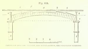
settling after the centres are withdrawn. The arches being thus secured, are afterwards levelled and filled up with a concrete of lime and ashes, on which is laid the flooring of tiles or stone flagging, as the case may be." The best and safest rise for arches such as now described is 11 inch for every foot of span.
