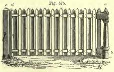
MILES' WOODEN FIELD-GATE WITH CAST-IRON HEEL-POST.
