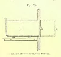
manger slides in and out on small pulleys on the bar a a; the projecting part b prevents it being pulled out too far.
