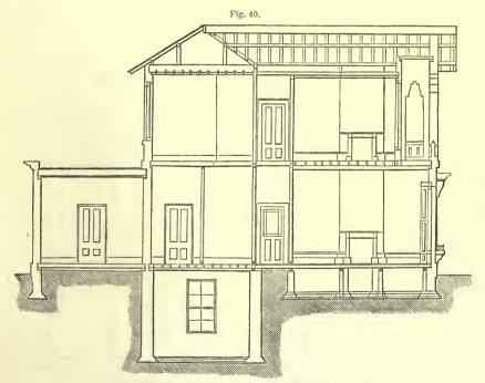
LONGITUDINAL SECTION IN THE LINE & B, FIG. 32-SCALE IN FIG. 32.
