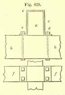
IRON SADDLE FOR JOINING BEAMS CROSS-ING AT RIGHT ANOLES-SCALE, & INCH TO THE FOOT.
