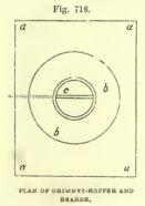
The brickwork of the flue rests on a a, which serves as a chimneybearer, thus obviating all necessity for using the dangerous material wood for this purpose. The hood or hopper b b tapers gradually upwards to the size designed for that of the flue. The upper part of b forms the throat of the chimney; if the flue is made of circu-
