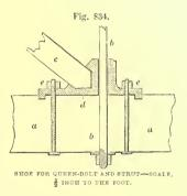
straining-beam and principal rafter: a is the queen-bolt, the head of which is sunk into a recess in the box or shoe b b, c the strainingbeam, d the principal rafter.
