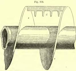
RAKE BETWEEN THE THREADS OF ARCHIMEDEAN SCREW CONVEYOR.
