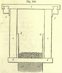
SECTION SHOWING ARRANGEMENT OF PARTS OF MOULD.
