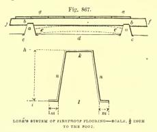
l 4 inches; breadth of flange  $m^{\frac{3}{4}}$ inch. The thickness of the sides  $n n \frac{8}{10}$  inch, of top k and flanges m m  $\frac{7}{20}$  inch. The width of the flat tiebars d is  $\frac{3}{4}$  inch, their thickness 13 inch.
