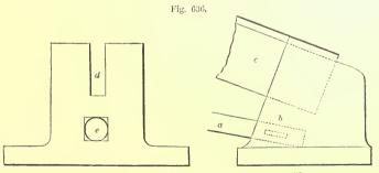
SIDE AND END ELEVATION OF RAFTER-SHOE-SCALE IN FIG. 657.
