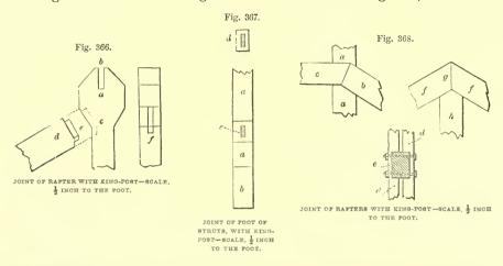
straining beam c butts immediately against the principal rafter b; the queenpost a a being bolted in two halves on d and d, embracing the beam e, and secured by bolts and nuts. In the same figure, f f represents the principal rafters butting at g; the king-post h being bolted in two halves as at d and d.
