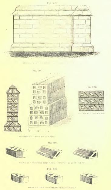
others just described. The form of brick shown to the right of fig. 204 is used for internal jambs and chimneys, and is  $8\frac{3}{4}$  inches long. The two other stretchers in this figure show how one or two angles may be chamfered in the process
