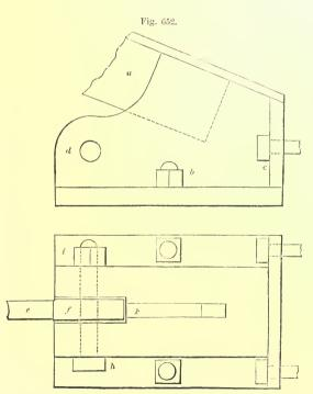
SHOE IN FLAN AND ELEVATION FOR SECURING FEET OF RAFTERS-SCALE IN FIG. 657.
