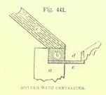
jecting piece e, or "cantaliver" as it is termed, may be, for roofs of ordinary size, 4 inches wide by 1 thick; the size of gutter inside may be from 3 to 4 inches wide and deep, inside measurement.
