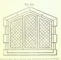
should run in horizontal, not vertical length. Good proportion for cottage window-lights are 4 feet high by 18 inches wide, or 2 feet 9 inches by 15 inches."
