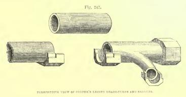
tory, Wottoon, Isle of Wight, or 150 Leadenhall Street, London) pipes, which are of the "butt joint" kind; "chairs" being used to connect the length of pipes. In fig. 248 we give views of the "chair." Mr Cooper states the advantages of his system to be as follows :—"They provide ready access to any part of the drain, for examination, without disturbing any other part, or point of the invert, of the drain. The pipe, being laid on the under connection, butts the adjoin-
