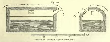
is provided at the end of the tank, which is always kept open, to allow of the ingress of air and the egress of the foul emanations. The crown of the arch
