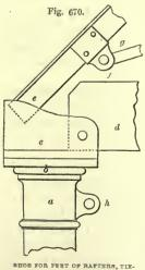
SHOE FOR FEET OF RAFIERS, THE-BEAM, AND THE-RODS-SOALE, 1 INCH TO THE FOOT.
