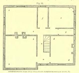
d d bedroom, 14 feet by 10; e servants' bedroom, 11 feet by 9; f linen-closet, 9 feet by 4 feet 6 inches; g water-closet, 6 feet 9 inches by 2 feet 6 inches. 338. Of this house we give front elevation in fig. 64.
