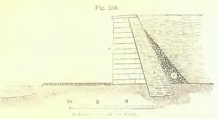
sions of the wall a, fig. 230, will be regulated by circumstances : if the height is 12 feet, the breadth at bottom should be 6, and at top 2. Every
