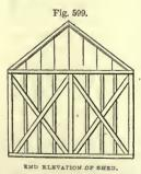
In fig. 597 we give plan of bark foundation for the shed. In fig. 598 side elevation, showing arrangement of timbers: a a door-spaces; b b upright posts and cheek-posts of door-spaces; c c roof-timbers; d d, e e braces. In fig. 599 we give end elevation. These walls are 12 feet high, but they would be sufficiently high at 9 feet.
