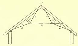
ROOF TRUSS OF OCTAGONAL SHED-SCALE, 1 INCH TO THE FOOT.
