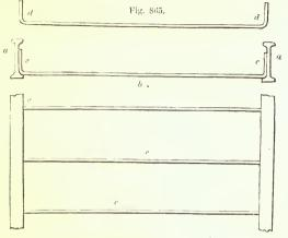
The floor is formed of flat arches of hollow bricks e e, springing from the sides of the girders. The joists f f are notched into the upper part of the girders b b. while the flooring-boards g g are laid in the ordinary method.
