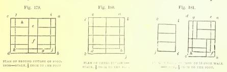
of the bricks in the course immediately beneath, just as shown in the section in fig. 177. Should a 9-inch wall be required, as shown by the dotted lines k m in fig. 177, the bricks will be laid as in plan i j k l, fig. 181; j i will correspond with h f, i l with f e, and j k with h g.
