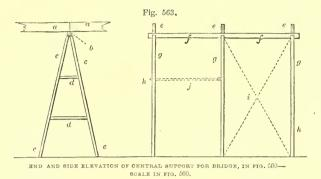
which may be used where the bridge, as in fig. 560, has not much pressure to support—as in the case of a foot-bridge—a a,  $e \ e \ c$  is the beam, corresponding to  $e \ e$  in fig. 561, resting on the cross-beam  $f \ f$  or b. This is supported by the stays  $c \ c \ c \ a$ three points  $g \ g \ g$ . The stays  $c \ c \ c \ a$
