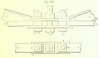
JUNCTION OF KING-BOLT, RAFTERS, AND THE-RODS-SCALE IN FIG. 657.
