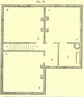
Ground-plan of a third-class farmhouse—scale,  $\frac{3}{16}$  of an inch to the foot.
