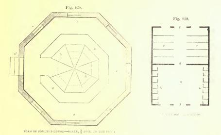
**1709.** In fig. 939 we give plan of poultry-house : a the feeding-place, b b the nests, c roosting-poles, d middle door, c back, and f front door.
