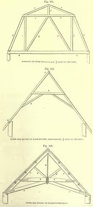
1222. High - pitched or Gothic Roofs.— In fig. 422 we give a truss for a high-pitched roof for a 20 - feet span; a a, 4 inches by  $3\frac{1}{2}$ ; b, 5 inches by 4; c,  $3\frac{1}{2}$ inches by 4.
