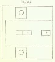
RAFTER-SHOE FOR ROOF IN FIG. 632-SCALE IN FIG. 657.
