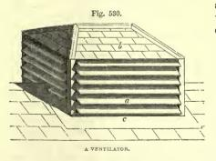
answer the double purpose of permitting the escape of heated air and effluvia, and of preventing the entrance of rain or snow. The blinds are covered and protected by the roof b, made of slates and lead; c is an apron of lead. Such a ventilator would be more ornamental to the steading than fig. 530 is, and more protective to the blinds, if its roof projected 12 inches over. One ventilator 6 feet in length, 3 feet in height in front, and 2 feet above the ridging of the roof, for every six
