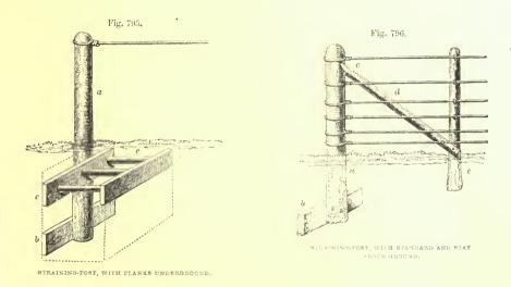
1546. A third method still is given in fig. 796, where a similar size of post a, to the others, is placed in the pit, 3 feet deep, having a piece of wood b, 2 feet long, 6 inches broad, and 2 inches thick, nailed to the back part of the bottom; e is a standard driven into the ground, at 4 feet distance, in a line with the
