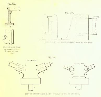
1522. Simpler modes of erecting the rails of this foot-bridge are illustrated in fig. 768, where a a shows one of the upright standards—of which as many
