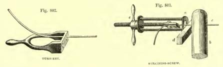
and under the wire c, a piece of wood d, about 2 inches square. It is necessary, before beginning to work the screw e, to place a temporary spur of wood to the inside of the post about b, which is removed when the next space is strained up, and so on, until the next extreme post is strained from.
