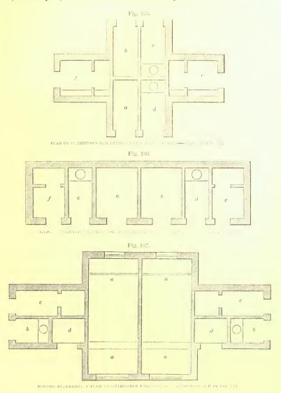
462. Outhouses for Two Double-Detached Composite Cottages, fig. 139: a a, a a coal-stores, each 4 feet by 6; b b, b b privies, each 3 feet by 6; c c, c c pigsties, 4 feet by 6 each. Alternative Plan, fig. 140: a a, a a privies; b b, b b coal-stores, 4 feet square; c c pig-sties, two at the ends of the coal-stores b b, not shown in the figure, 4 feet by 6.
