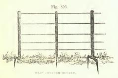
as to present its flat side to the pressure. The horizontal bars—in the majority of instances round, but in some cases square, set diagonally—are "tannered" at the ends by machinery, which takes off the least possible proportion to form a shoulder for riveting them to the uprights.
