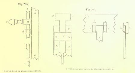
downwards by the rack, see fig. 705, the cross passes into the space, and the window is secured : simultaneously, the bolt e of the lower part of bar b, fig. 706, is passed into its catch. In fig. 707 the bar c slides in a brass stud f, secured to the window-stile g, corresponding to a a, fig. 704; d e being the cross.
