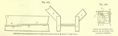
1237. Roans or Gutters cut out of a Solid Block of Wood .- Fig. 446 represents a
