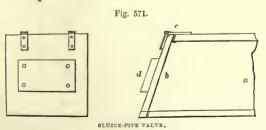
1353. In fig. 571 we give a sketch illustrative of a form of sluice-valve; a the box, b the valve, hinged at c. A piece of iron d, may be bolted to the back of the valve to keep it closed. The figure to the left is a front view of valve. An *iron* sluice-valve will be found illustrated in
