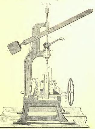
POWIS' MORIISING, TENONING, AND BORING MACHINE IN PERSPECTIVE.
