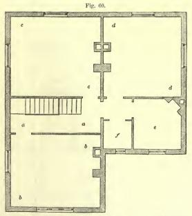
plan, and in fig. 60 chamber or first floor plan, of a two-storeyed farmhouse. The scale to which these plans are constructed is  $\frac{1}{16}$  of an inch to the foot.
