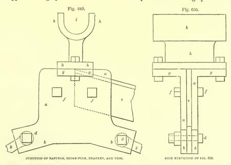
1433. We give in fig. 651 the elevation of another method of joining the assemblage of parts shown in figs. 649, 650, where a a is the cast-iron shoe, bthe recess for ridge-pole, c the rafter, d e the line of tie-rods e c, fig. 645, of which f f, fig. 651, is a side elevation, and g g edge, showing part which embraces the shoe a a.
