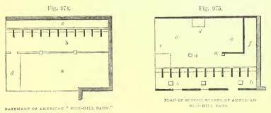
stalls, 3 feet 3 inches by 8 feet; c the feeding-passage, 4 feet 6 inches wide; the part d is paved. In fig. 975 we give the plan of second storey, in which a a are the posts supporting hay-floor over stable-passage, b b cattle-stalls, c c haymow or balk, d the hay-shoot or funnel, e another funnel, f passage. In fig. 976 we give a perspective elevation of the barn.
