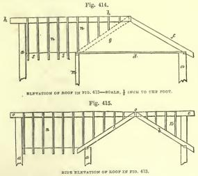
n n the rafters corresponding to those marked f f in fig. 413. In fig. 416 is the arrangement of timbers at c c, fig. 413, drawn to a larger scale; a a part
