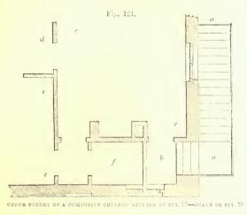
442. In fig. 125 we give part plan of cottage over that in fig. 117: a a outside stairs; b porch; c pantry; d bed-closet over d in fig. 117; e e living-room; the scullery and bed-closet correspond in size and position to apartments marked b and c in fig. 117.
