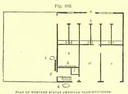
through which to pass the manure from time to time; c is the corn-crib. The floor of this, as well as the corn-cribs in the stalls, indicated by the small black circles, should be from  $2\frac{1}{2}$ to 3 feet above the level of the ground, so as to admit of the pigs getting beneath them. By this arrangement, not only will shelter be provided for them, but they will be enabled to pick up all scattered corn, and also prevent rats from accumu-
