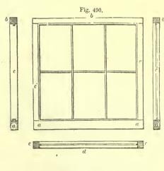
ELEVATION AND SECTION OF SASH-FRAME OF WINDOW.
