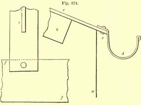
GUTTER'OF IRON ROOF-SCALE IN FIG. 657.
