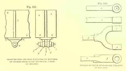
twice the size of the detail in fig. 842: a is the end of the horizontal truss rod g in fig. 841, with its circular head and bolt hole b; c is an edge view
