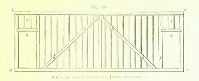
1186. In fig. 385 the partition is adapted to a 22-feet span: the head a b, 6 inches by 6; the sill c d, 6 inches by 4; the tie-beam c e, 6 inches by 5;
