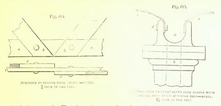
1472. In fig. 685 we show a mode of connecting corrugated arched iron plates c and c with the gutters a, which are either bolted to the cap of column b
