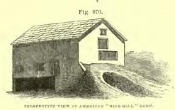
posts 20 feet above the basement; the roof steep, which gives more room for hay, is more durable and stronger if left without purlin support; two middle cross works, which make the girts 13 feet. It is situated on a somewhat steep side-hill, facing the south-east; the basement wall on the north side, and the west part of the south side to the west middle cross work, 8 feet high. The
