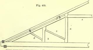
TRUSS WITH TWO QUEEN-POSTS FOR 47-FEET SPAN-SCALE, & INCH TO THE FOOT.
