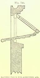
value a is hinged at b b, the staple or bar passing through the eyes of two studs leaded into the wall. The form of ventilator, fig. 292, as Looker's ventilator, is also made in cast-iron, and is well adapted for stables. The forms illustrated in figs. 528 and 529, may also be used for admitting and regulating the supply of fresh air. In fig. 744 we give a section of
