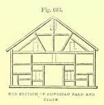
States; with extreme lightness it possesses great strength. All mortise holes, tenons, auger holes are avoided in the construction, thus insuring the perfect integrity of the timbers. Nails alone are used in the manner hereafter illustrated, and advantage taken of the full tensile and compressible strength of the timber. For the following illustrations and descriptions, we are indebted to the *American Cultivator*.
