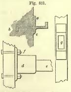
CAST-IRON SHORS FOR "JOISTS," " WALL-PLATES "-BCALE, 1 INCH TO THE FOOT.
