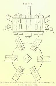
1464. Gutters for Iron Roofs—Gutter for Single Roof.—In fig. 674 we illustrate a method of forming the gutter of an iron roof, in which a is the wall on which rests the shoe for rafter b. The flange c of the rafter b is continued past the butting end c, and carried outward beyond the wall a. The zinc or
