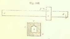
ELEVATION AND SECTION OF GAUGE-SCALE, & INCH TO THE INCH
