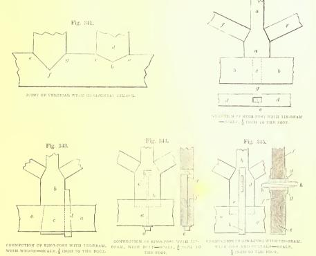
tion is made by passing an iron strap b b, round the tie-beam a a, and connecting it to the king-post c d by the keys h h, and cottars g g—these passing through an aperture cut in the king-post and slots in the sides of the strap b b. In the section, f f is the king-post, e the tie-beam.
