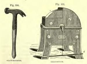
1660. Grindstone. -In fig. 891 we illustrate a convenient and cleanly form of grindstone, the framing a a of which is of cast-iron. The stone is covered with a casing b b, leaving part only of the stone exposed, as at This arrangement с. prevents the water from being scattered about. The revolution of the stone is caused by the action of the foot of the operator on the pedal
