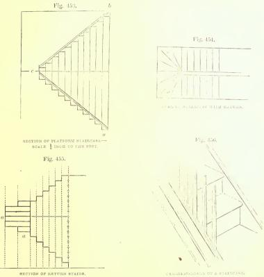
1245. Laying out of the Steps on the Notch-Board.—We now proceed to explain another way of laying out the positions of the treads and risers, on what are termed "string" or "carriage boards"—as  $a \ b \ c \ d$ , fig. 457, where  $e \ f, \ g \ h$
