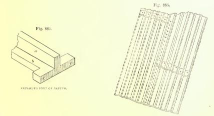
JOINING CORRUGATED PLATES OF ZING TOGETHER.
