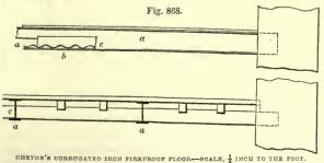
1639. In fig. 868 we give a system of fireproof flooring patented by Mr C. Cheyne, C. E., 34 Great George of Street, Westminster, London, in which malleable iron corrugated plates are used in conjunction with iron beams and concrete filling in. "Fig. 868 is a section section of same. The
