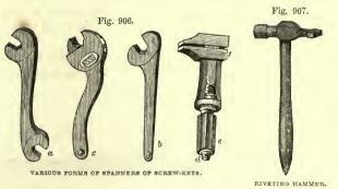
warrous forms of keys manufactured by Ibbotson & Co., Birmingham:  $a \ b$  are keys to embrace nuts of determinate sizes. Keys, or shifting spanners, are shown at  $c \ d$ ; by turning the handle e a screw is operated upon, by which the jaws fare made to recede from, or approach to, each other, as desired.
