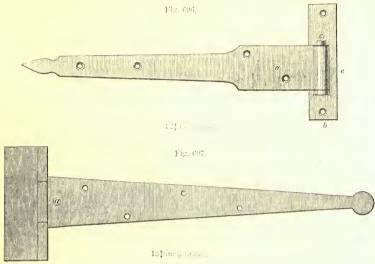
diameter. In fig. 697 the length of hinge is  $13^3_1$  inches, the breadth at part a  $2\frac{1}{4}$  inches; the length of cross  $4\frac{3}{4}$  inches, and breadth  $1\frac{3}{4}$  inch. Fig. 698,
