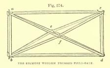
a pavilion roof. A similar truss is formed for the other face of the gate, whose apex is at f. Through the points e and f, the apeces of the trusses, passes the iron bolt e f, the head of which holds the bars at f; and a screw and nut upon a plate hold those at e; and when the screw is tightened, the trusses are brought nearer together in the centre, and their ends abut with great force against the angles of the rectangular
