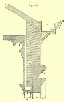
BECTION OF WALL SHOWING GUTTER WITH CANTALIVER-BOALE,  $\frac{1}{2}$  INCH TO THE FOOT.
