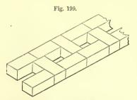
14-INCH HOLLOW WALL-SCALE, 1 INCH TO THE FOOT.
