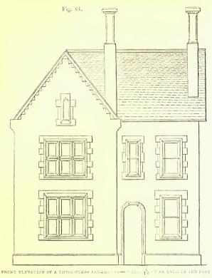
335. Second Design for a Third-Class Farmhouse.-In fig. 62 we give groundplan, and in fig. 63 chamber-plan, of another two-storeyed small farmhouse.
