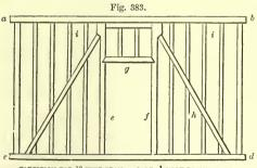
PARTITION FOR 18-FEET SPAN-SCALE, & INCH TO THE FOOT.
