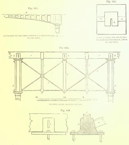
ELEVATION AND SECTION OF SHOE-SCALE, I INCH TO THE FOOT.
