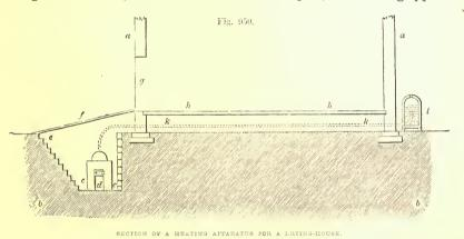
the arrangements of which will of course differ in different localities. Fig. 950 is a longitudinal vertical section of a drying-house :
