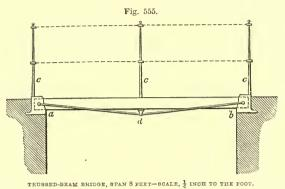
bridge for a span of 8 feet. The beam rests in castiron shoes a b; c c c are the hand-rails, and a d bis the malleable-iron truss. In fig. 556 is a sketch showing the arrangement of trussed beams for a span, of 32 feet, divided into two spans of 16 feet each. The beams a a, 12 inches by 8, rest at the ends b b on the retaining walls; the other ends
