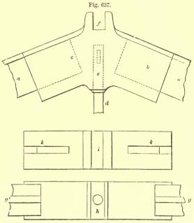
ELEVATION AND PLANE OF SHOE FOR UPPER END OF RAFTER-SCALE IN FIG. 657.
