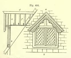
ELEVATION AND SECTION OF DORMER WINDOW-SCALE, & INOH TO THE FOOT. 1232. Gutters.—Where the rafters project over the wall—which in the majority of the simpler constructions will be the case—the manner of making the gutters in a variety of ways is shown in the following figures: In fig. 437,
