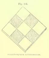
when partly consolidated, throw on another layer of stones, and above this another of the tar and sand. When the upper is nearly consolidated, but not hardened, place the flat tiles, beginning at one end, and advancing in such a manner as to leave no footsteps on the soft material. Instead of tar and sand,
