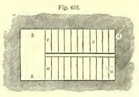
PLAN OF PLATFORM STAIRS-SCALE, 1 INCH TO THE FOOT.
