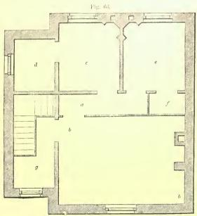
CHAMBER-HOOR PLAN OF A "URD-CLASS FARMHOUSE-SCALE IN FIG. 07
