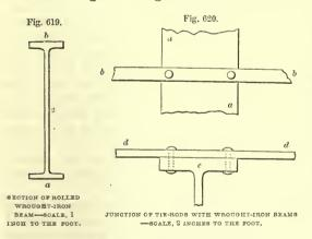
rails, adapted for wroughtiron fireproof construction; the length *a b* being 20 feet. The width of bottom flange is 4 inches, and thickness  $\frac{1}{2}$  an inch; of top flange, 4 inches, and thickness  $\frac{3}{4}$ inch; the thickness of rib  $c \frac{3}{8}$ ; total depth of beam 15 inches.
