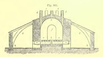
TRANSVERSE VERIICAL SECTION OF DRAIN-TILE HILN.
