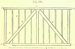
the posts d d d d d, 4 inches by 3; straining-beam e, 4 inches by 4; struts or braces f f, 4 inches by 3; g filling-in pieces, 4 inches by 2.
