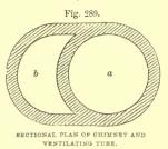
King Street, Manchester. By the use of these double tubes, much brickwork in the chimneybreasts is saved; and where this is of importance, as in brick buildings, the projection being less, a little extra space is added to the room. Where single chimney-flues are run up separately, double tubes of an elliptical form, as in fig. 289, might be used. The chimney-flue would thus be completely circular; the shape of the ventilating flue would be slightly irregular, but in nowise calculated to
