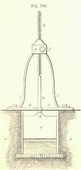
ELEVATION OF IRON SLUICE VALVE AND RACK-SCALE } INCH TO THE FOOT.
