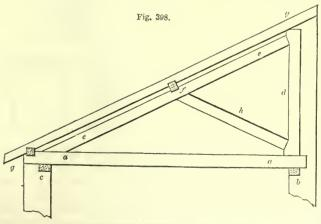
of roof; this is called a "lean-to," and is adapted for covering cart-sheds, &c. The form in fig. 397 is calculated for spans of from 10 to 12 feet. The scantling of the rafter or beam b c is 105 inches by  $2\frac{1}{2}$ ; the wall-plate b, 4 inches by 3. The joists should project 18 or 20 inches beyond the lower wall d, as at f, and should be placed on the walls
