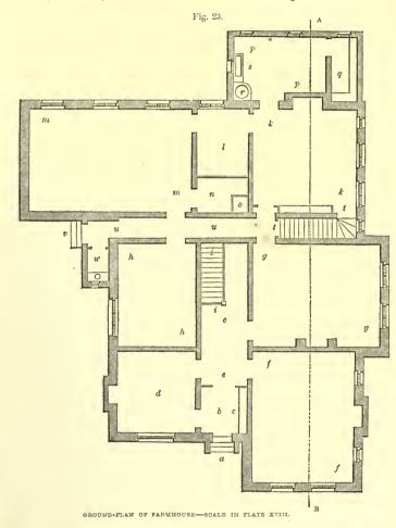
which articles are conveyed to the cheese-room above; p p scullery, 14 feet by 8 feet 6 inches, with pantry q, wash-boiler r, and slop-stone s. The back stairs to servants' bedroom are at t t; u u a passage, 3 feet wide, leading to back-entrance v; w a water-closet, 3 feet 6 inches wide.
