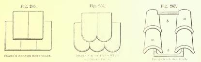
*a* to cover the joints of the flat tiles b; price of *a*, 9d. per pair; price of *b*, £10 per 1000. In fig. 268 we give a diagram of Peake's quoined valley, and in fig. 269 of hip-tiles. Price of fig. 268,  $3\frac{3}{4}$ d. each; of fig. 269,  $4\frac{1}{2}$ d. each. In fig. 270 we give a diagram of ridge-tiles, and in fig. 271 grooved ridge-tiles, in the groove *a* of which the ornamental tiles shown in fig. 272 are fitted.
