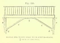
1342. Trussed-Girder Bridges.-In fig. 555 we give an elevation of a girder
