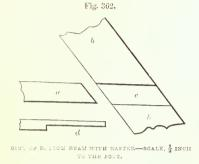
JOINT OF RAFIER WITH THE-BEAM-SCALE, 1 INCH IO THE FOOT.
