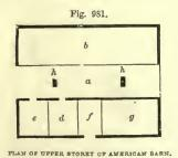
stalls is the passage i i, for the cattle as they pass in and out of their stalls. The stable doors m, are six in number. In this barn, accommodation is given for fiftysix grown cattle in twenty-eight double stalls, with room for twenty to thirty calves in the end stables. Storage for 150 tons of hay is also provided.
