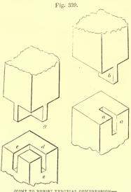
JOINT TO RESIST VERTICAL COMPRESSION-SCALE, 1 INCH TO THE FOOT.
