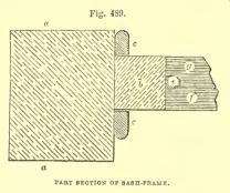
to the foot. The lower rail a a, is 3 inches by 2; the upper, b, 2 inches by 2, as also the side ones c c. The section to the right shows position of top and
