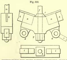
JUNCTION OF MING-BOLT, STRUTS, RAFTERS, AND THE-RODS-SCALE IN FIG. 657.
