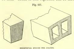
already pointed out, in Section Third, as necessary to be attended to in constructing arched work. The objection is, however, wholly met by the use of the radiated bricks, of which, in fig. 237, we illustrate one or two forms. These are now manufactured at a price very little above that of ordinary bricks, and suited for conduits of various sizes. These bricks require less cement than ordinary ones, and give per-
