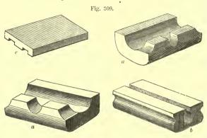
drainage bricks for the floor of stables, byres, &c., manufactured by H. Clayton, Aslar Works, Dorset Square, London. In fig. 309 a and a are gutter bricks, b a drain brick, and c a cover for gutter. In fig. 310 we give a diagram showing the floor of flushed pavement, with the gutter partly uncovered, to show its connection with the pavement.
