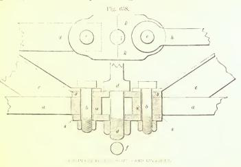
king-bolt passes through the central aperture i, and the whole are secured by the bolts b b passing through the holes e e.
