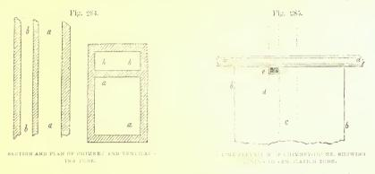
is made at e, communicating with the interior of the ventilating flue, the upward current therein will withdraw the vitiated air from the room through the aperture e, which may be covered with an ornamental grating, as in fig. 286.
