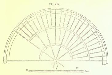
PART PLAN OF TRUSS OF ROOF FOR THRASHING-MILL HORSE-WALK.
