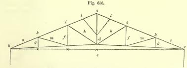
SEELETON OF TRUSSED ROOF 30 FRET SPAN-SCALE IN FIG. 657.
