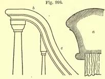
ELEVATION AND SECTION OF HANDRAIL.
