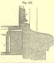
PART SECTION OF BASE OF BAY WINDOW-SCALE, 1 INCH TO THE FOOT.
