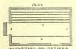
house, of timber with brick basement, which may be made of any desired length, and divided into departments for varieties of birds : a steps up to floor, b space occupied by nests, d roosting-place, c floor. In fig. 936 is the front elevation, and in fig. 937 section; in this, a the nests, b the roosting-place.
