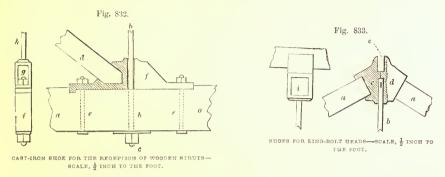
support of the principal rafters: a a are the upper ends of the rafters, b the king-bolt, c d the box, the side c of which is in section, the side d in elevation. An aperture is cast through the solid part to admit of the king-bolt b being passed through; the ridge-pole passes into the recess e; i shows a front view of the rafter-box.
