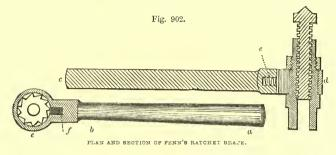
placed within the bar of iron a b; a slot is cut in the lever to admit of the sliding catch f. The greater the strain on the lever the more closely does the catch engage with the catchwheel e, and which is driven up by a
