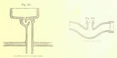
1109. Fig. 295 shows form of syphon-trap adapted for sinks and sculleries; and in fig. 296 a trap or cesspool for house-yards.
