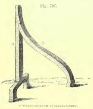
quired. The extreme posts require a stay b in addition, which costs according to its weight. The cost of such a straining-post is this :—
