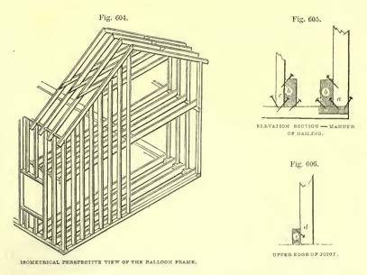
1381. The sizes of the different pieces of timber in a frame of this size are: sills, 3 inches by 8; corner studs, 4 by 4; other studding, 2 by 4; plate, 1 by 4; side strips, or side girts, 1 by 4; rafters, 3 by 6, or  $2\frac{1}{2}$  by 5 will do; collars, 1 by 4; floor joists, 3 by 8, or maybe 2 by 7. Rafters, studdings, and joists are 16 inches between centres.
