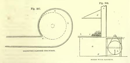
adapted for the use of the fanners is shown: the wheel for giving motion to the fan is fixed on a frame f, at the back of the forge, on the top of which the fan is placed. The large wheel is put in motion by a treddle g and connecting-rod h,
