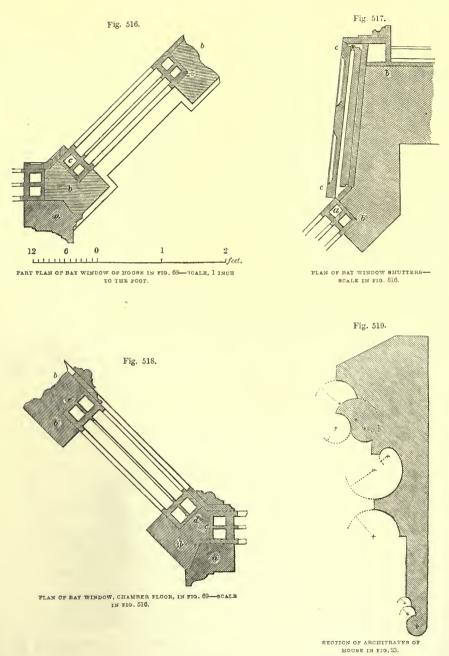
1278. Architrave.--In fig. 519 we give section of mouldings of architrave for house in fig. 23.
