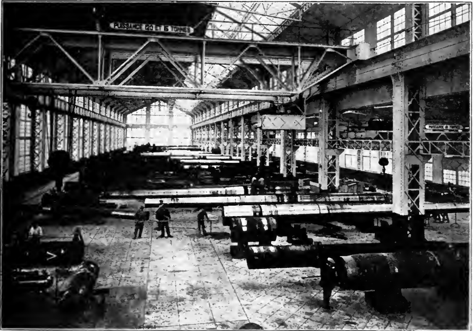
TESTING THE BORES OF GUNS IN A FRENCH ARMAMENT PLANT
