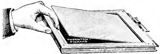
Fig. 125.—LAYING PLATE IN AMERICAN PATTERN SLIDE.
