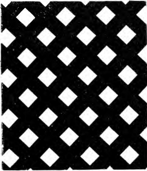
Fig. 893.—MAGNIFIED APPEARANCE OF HALF-TONE SCREEN.
