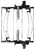
Fig. 500.—SECTION OF DOUBLE MENISCUS LENS.
