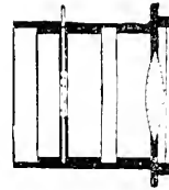
Fig. 499.—SECTION OF SINGLE NON-ACHROMATIC LENS.
