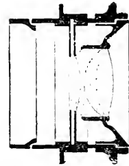
Fig. 512 —SINGLE COMBINATION OF ORTHOSTIGMAT USED SEPARATELY.
