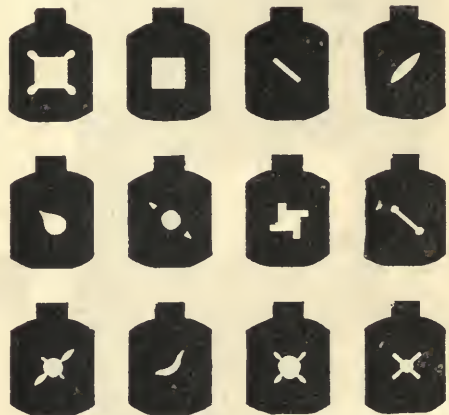
Fig. 894.—DIFFERENT SHAPES PROPOSED FOR HALF-TONE STOPS.
