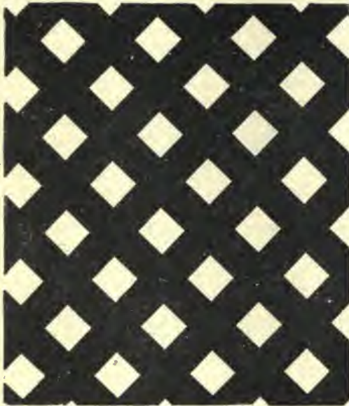
Fig. 893.—MAGNIFIED APPEARANCE OF HALF-TONE SCREEN.
