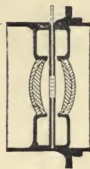
Fig. 506.—SECTION OF WIDE-ANGLE RECTILINEAR LENS
