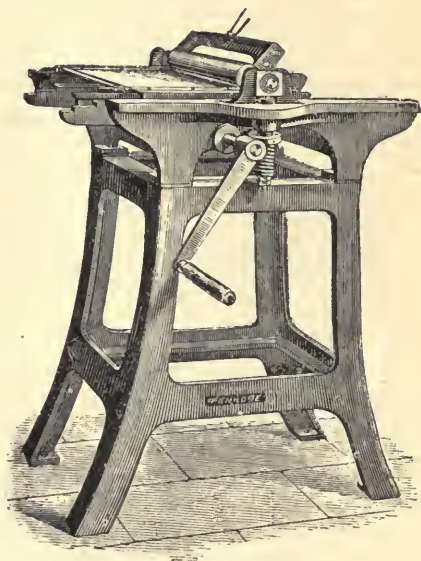
Fig. 888.—COLLOTYPE PRESS, WORKING WITH ROLLER AND ECCENTRIC.
