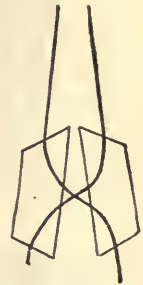
Fig. 741.—PATH OF RAYS THROUGH BINOCULAR PRISMS.
