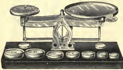
Fig. 18.—COUNTER SCALES AND WEIGHTS AND APOTHECARIES' SCALES AND WEIGHTS.
