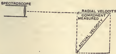
Fig. 810.—DOPPLER'S PRINCIPLE APPLIED TO MEASUREMENT OF VELOCITY.
