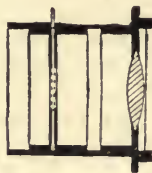
Fig. 499.—SECTION OF SINGLE NON-ACHROMATIC LENS.
