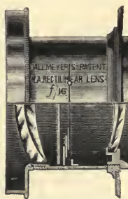
Fig. 507.—DALLMEYER WIDE-ANGLE RECTILINEAR LENS.
