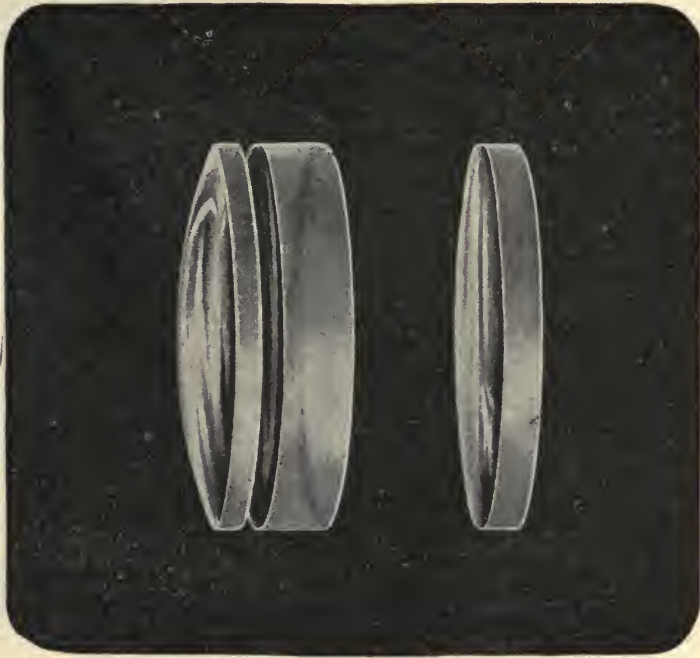
Fig. 551.—THREE SIMPLE GLASSES OF COOKE LENS.
