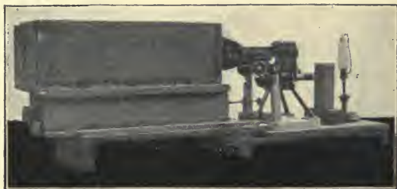
Fig. 736.—SIMPLE PHOTOMICROGRAPHIC APPARATUS.
