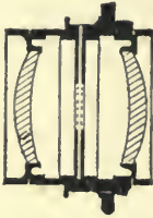
Fig. 500.—SECTION OF DOUBLE MENISCUS LENS.
