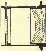
Fig. 502.—SECTION OF THREE-GLASS SINGLE ACHROMATIC LENS.
