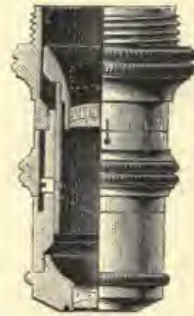
Fig. 692.—ZEISS OBJECTIVE WITH CORRECTION COLLAR.
