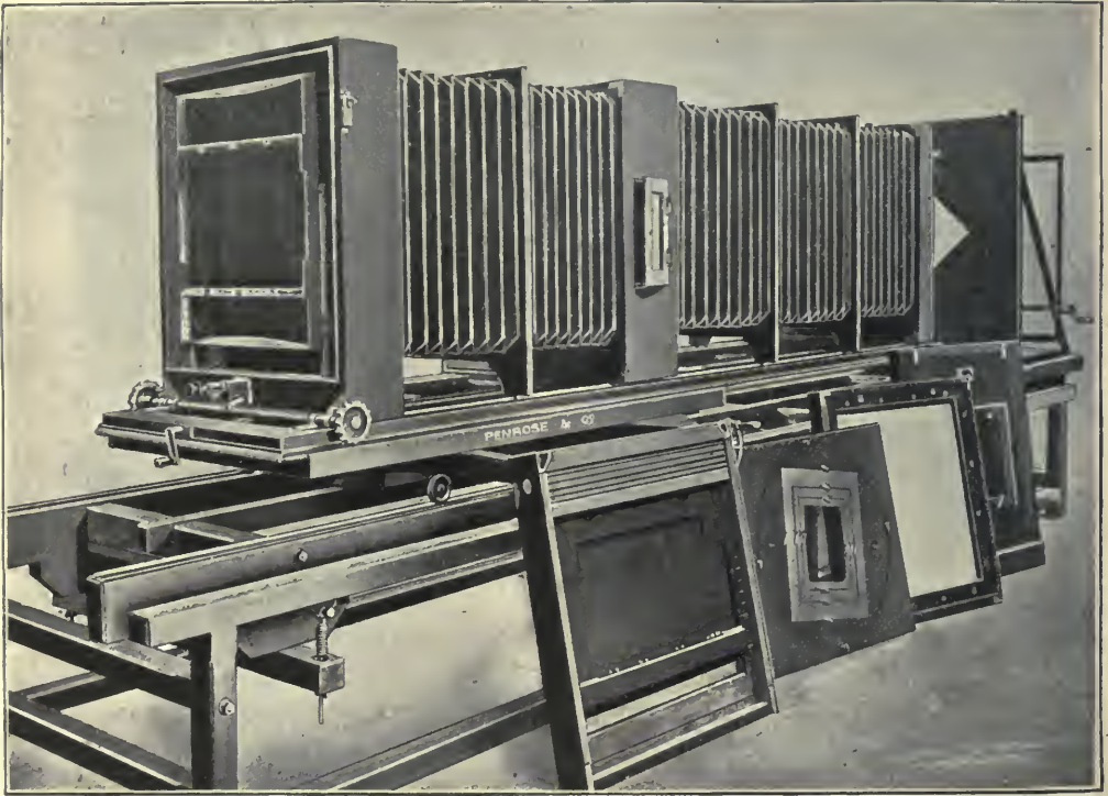
Fig. 899.—REPRODUCTION CAMERA WITH TRANSPARENCY EXTENSION.
