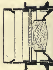
Fig. 512.—SINGLE COMBINATION OF ORTHOSTIGMAT USED SEPARATELY.
