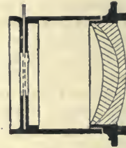
Fig. 501.—SECTION OF TWO-GLASS SINGLE ACHROMATIC LENS.
