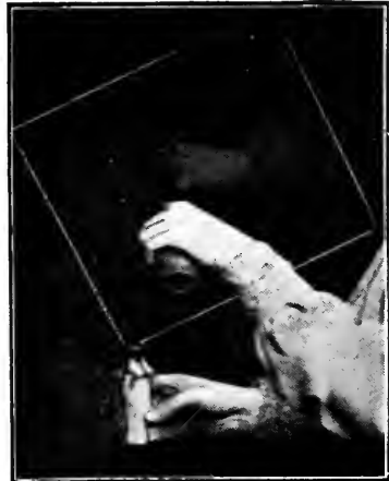
Fig. 145.—POURING OFF THE SURPLUS EMULSION.
