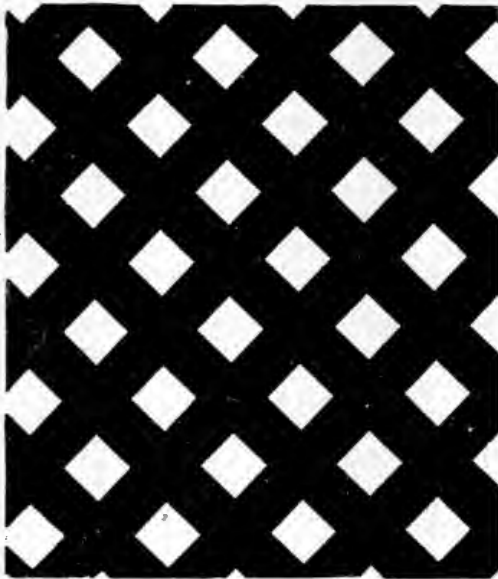
Fig. 893.—MAGNIFIED APPEARANCE OF HALF-TONE SCREEN.
