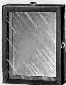
Fig. 374.—CELL FOR BICHROMATE LAMP.
