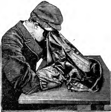
Fig. 642.—CHANGING BAG WITH RUBY EYE-PIECES AND WINDOW.
