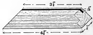
Fig. 90.—PIECE OF DARK-SLIDE FRAMING.
