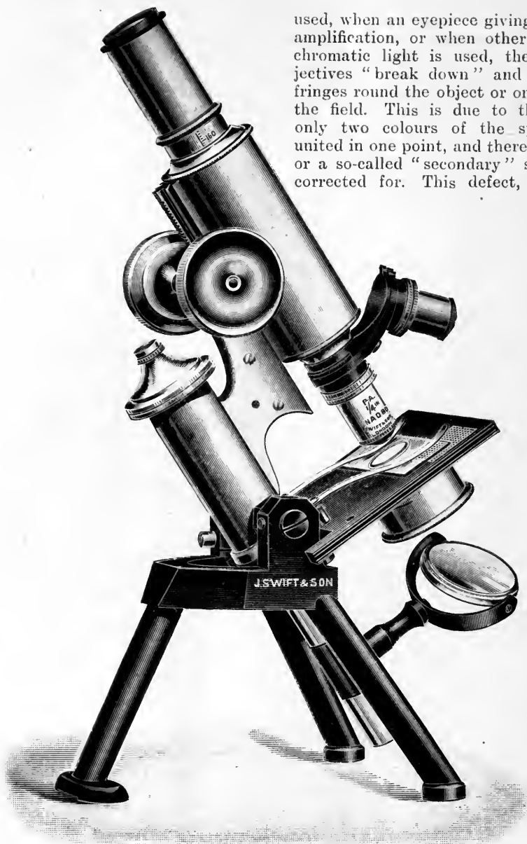
Fig. 691.—SWIFT'S STUDENT'S MICROSCOPE.
