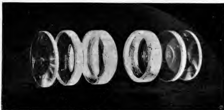
Fig. 513.—SIX COMPONENTS OF BECK-STEINHEIL ORTHOSTIGMAT.
