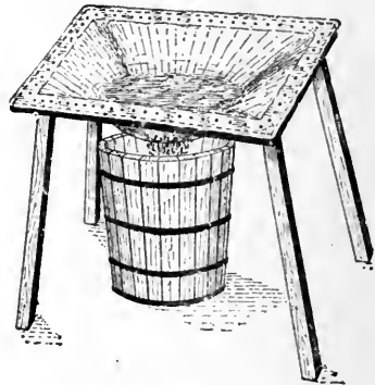
Fig. 882.—ARRANGEMENT FOR FILTRATION.
