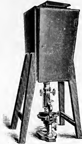
Fig. 730.—VAN HUERCK'S VERTICAL CAMERA.
