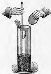
10. — Arrangement of apparatus to show that carbon dioxide is given off by germinating seeds.
