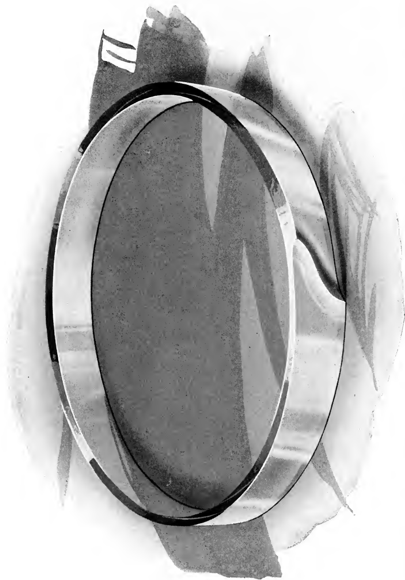
Prismatic ring (band ring type). In rotation, gives oscillation to a beam of light passing therethro.
