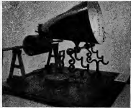
Mr. Scott invents first machine for recording speech 1866
