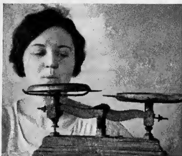
Blowing gently across the top of the over-turned scale pan will lift it
