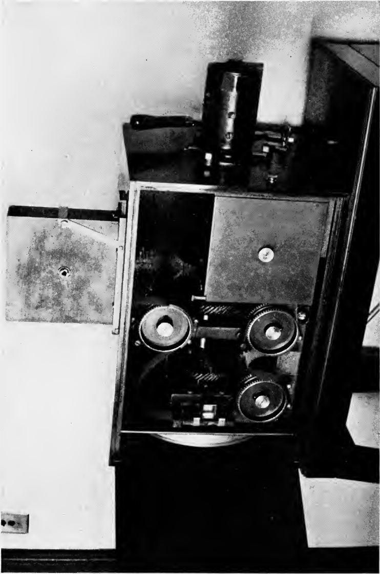
Chronotone camera in which motion pictures are made 3,200 exposures per second, later to be projected 16 pictures per second for study 200 times slower than taken.
