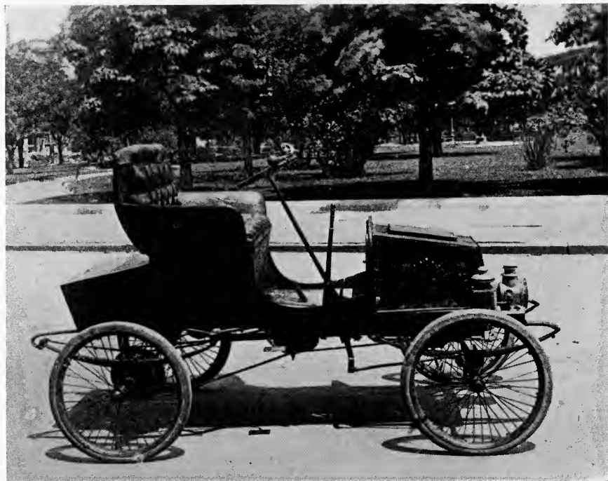
This horseless carriage is thought to be the first to have the engine under the hood in front.
