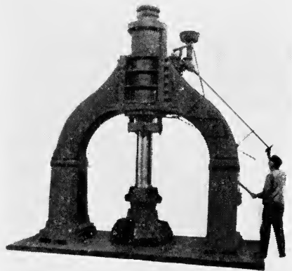
This hammer strikes a 3-ton blow
