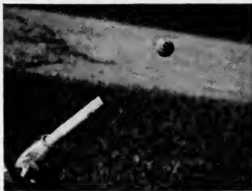
Showing how stream of air at 45° will hold ball suspended above ground
