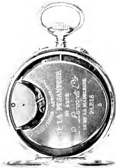
Watch showing a modern attempt to produce a self winder, which answers the purpose and is simpler than the Breguet type.
