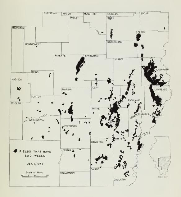
Fig. 2. - Illinois oil fields that have salt water disposal wells. The wide distribution of subsurface brine disposal is illustrated by comparison of the two maps. The 90 or so fields shown above have 86 percent of the total oil field area and 88 percent of the total oil production. If any fields have been inadvertently omitted from this survey of brine disposal, these two percentages should be correspondingly increased.
