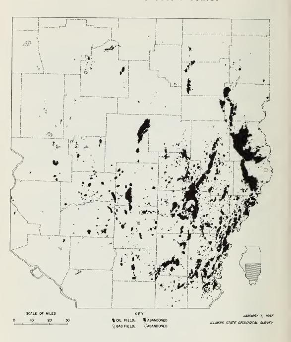
Fig. 1. - Oil and gas fields of Illinois except for a few that are outside of the area mapped. Illinois has about 370 oil fields, including abandoned fields. All but about 27 of them have been developed since 1937.
