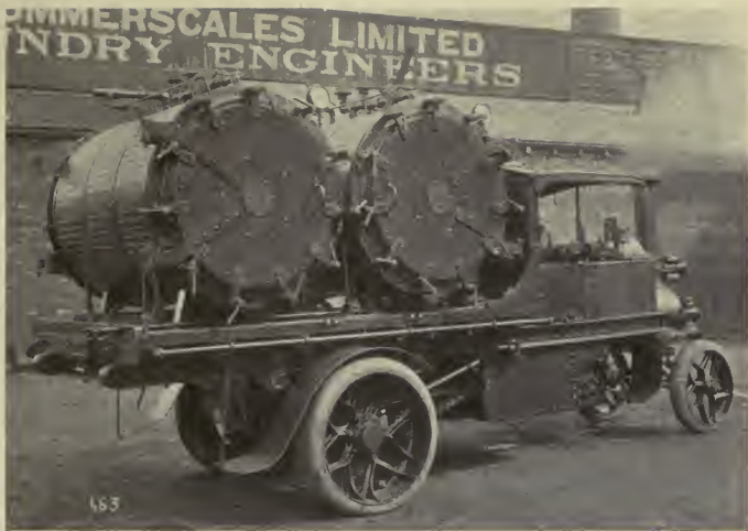
Disinfectors mounted on a steam lorry. Sent to France by the Order of St. John for use of a British Regiment.
