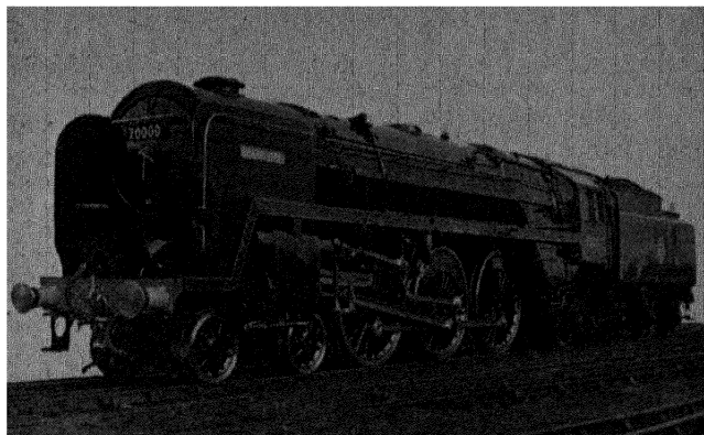
The first of the British Railways standard 4-6-2 Pacific locomotives, "Britannia" (no. 70,000), which was introduced into service in 1951.
