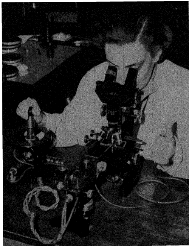
A machine enabling intricate surgical operations to be performed on living organisms less than 0.0001 in. long, which in 1951 was used at St. Mary's hospital, London.
