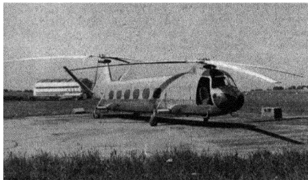
The Bristol 173, Britain's first twin-engined helicopter, which was designed to carry 12-14 passengers. The helicopter flew for the first time on Jan. 3, 1952.
