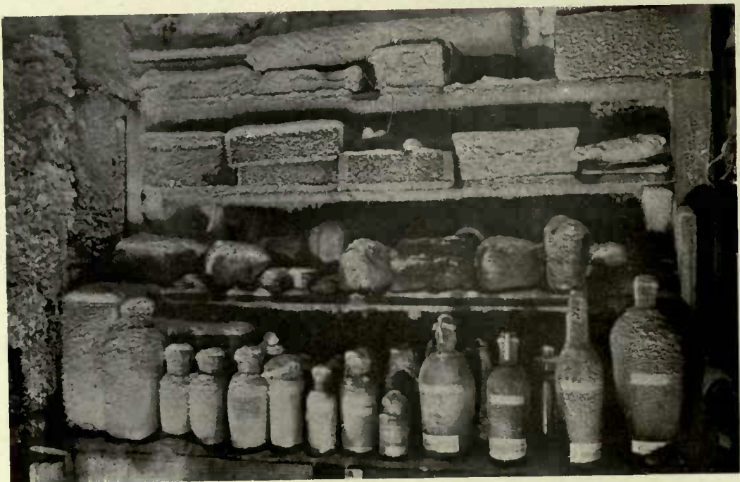
FIG. 2. A DISTANT VIEW OF THE CRUST OF PLATY ICE FORMED ON THE LABORATORY WALL
