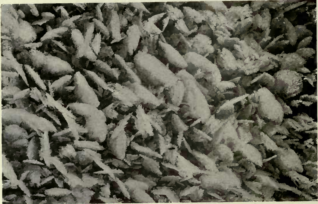
FIG. 1. A CRYSTALLISATION OF PLATY ICE ON THE LABORATORY WALL VIEWED AT A DISTANCE OF TWELVE INCHES
