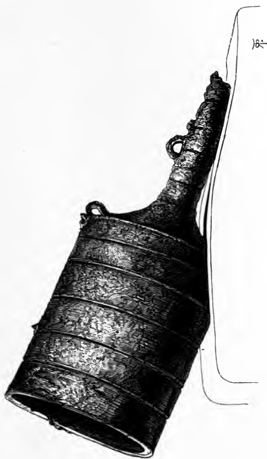
Wrought-iron Bombard, from Bodiam Castle; now in the Rotunda, Woolwich. Length of cylinder muzzle to touch-hole, 22 in.; total length, 44 in.; diameter, 15'4; weight, 6 cwt.
