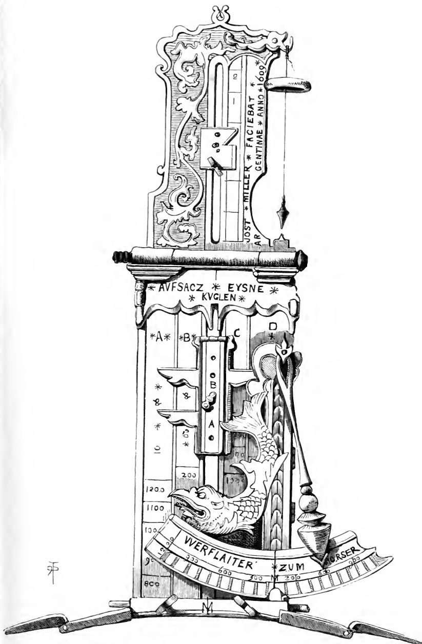
Tangent Sight for Cannon, made in 1609 by an Englishman. The plumb-line at the top shows the verticality of the Cannon. The little quadrant at the side the angle of elevation. A, B, C, D shows the elevations for 10, 20, 30, 40 pounders up to 1,200 yards. The sights are aperture-sights, as lately used in rifles. (In the possession of Mr. R. T. Pritchett, F.S.A.)
