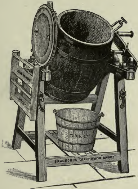
FIG. 30.—PERFECTED DIAPHRAGM CHURN
