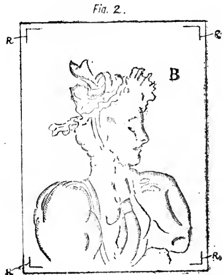
"Fig. 2 is a back view of the block with the embossing mould and register marks.
