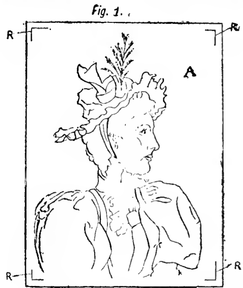
"Fig. 1 is a view of a photographic negative with guide or register marks thereon.
