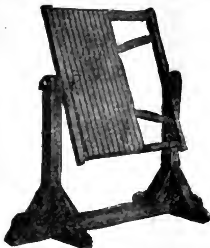
Fig. 3.—Wooden Developing Frame on its Winding Stand.
