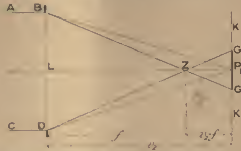
Fig. 5.—Illustrating formation of image of object at distance of sharp focus when obtaining infinity in "focus." P_1 is the sharp image on the focusing screen KK , of an object at such a distance that a point in an object at infinity is rendered on the focusing screen as a disc GG of the admitted diameter c . The distance of the object is
