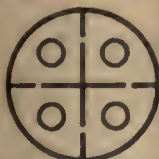
Fig. 6—Reversed diagram of cross-wires, the breaks in the lines and centres of dots are scraped away with a needle.
