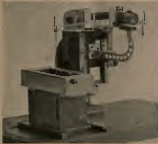
Fig. 9.—Auxometer for measuring thickness of gelatine film
