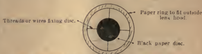
Fig. 7—Diagram of lens cap for testing for spherical aberration.
