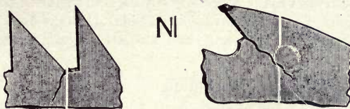
Cracks from Angular Filing
