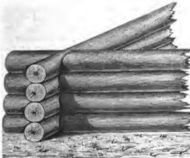
Fig. 1907. Blockwand.
