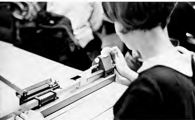
Managing a machine that measures the number of twists in a piece of thread is an intricate part of fabric study.
