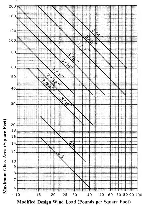
This chart is based on minimum thicknesses allowed in Federal Specification DD-G-451b
