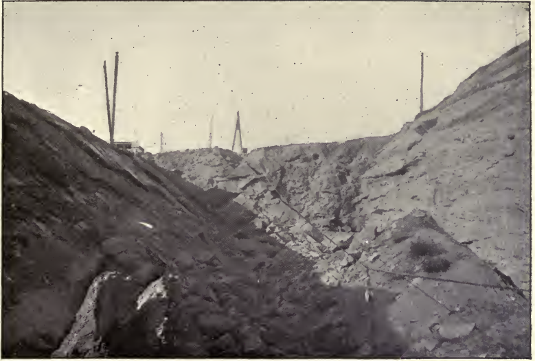
VIEW IN QUARRY NO. 1, HUMMELSTOWN BROWN-STONE COMPANY. Showing dip of strata and method of working.
