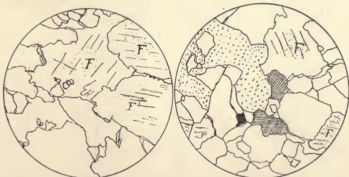
Fig. 7.—Micro-drawings of the Lumberville stone. F is feldspar, the clear areas quartz, the cross-lined areas clay and granular quartz, the dotted area calcite. Magnified 44 diameters.
